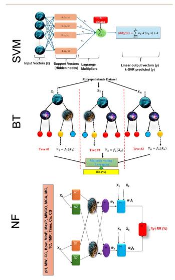
Scheme 1 Schematic of SVM, BT and NF model structure.
