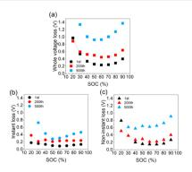
Fig. 2 (a) Whole voltage loss, (b) instant loss, and (c) non-instant loss of the cells with different cycle numbers.
