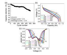
Fig. 1 Capacity retention (a), discharge (b) and relative  $d\Omega/dV$  curves (c) with varying cycle numbers for the pouch cell.
