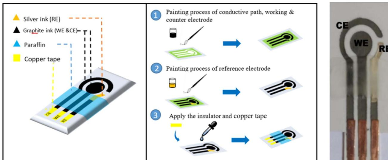
Fig. 1 The simple fabrication of various kinds of SPE for various applications. Three electrodes (working, counter and reference) were printed.<sup>13</sup> Similarly, gold, platinum and graphite coated working SPEs are also can be prepared with three electrodes configurations.
