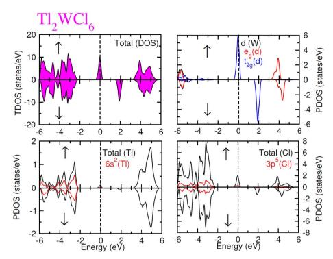
Fig. 4 Total DOS and partial DOS for DP Tl<sub>2</sub>WCl<sub>6</sub> and Tl, W and Cl ions in spin-up (↑) and spin-down (↓) channels by utilizing mBJ potential.
