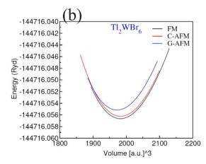
Fig. 2 Plots of volume optimization for DPs (a) Tl<sub>2</sub>WCl<sub>6</sub> and (b) Tl<sub>2</sub>WBr<sub>6</sub> in FM, C-AFM and G-AFM phases.
