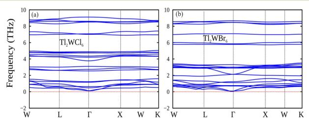
Fig. 8 The calculated phonon dispersion plot for DPs (a) Tl<sub>2</sub>WCl<sub>6</sub> and (b) Tl<sub>2</sub>WBr<sub>6</sub>.
