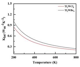
Fig. 7 The calculated lattice conductivity  $(k_{\rm lat}/\tau)$  for DPs Tl<sub>2</sub>W(Cl/Br)<sub>6</sub> against temperature 200–800 K.
