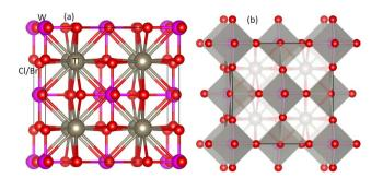
Fig. 1 Unit cell of DPs  $Tl_2WCl/Br_6$  (a) ball-stick model and (b) polyhedral model. Tl, W, and Cl/Br ions are represented by gray, pink and red spheres respectively.
