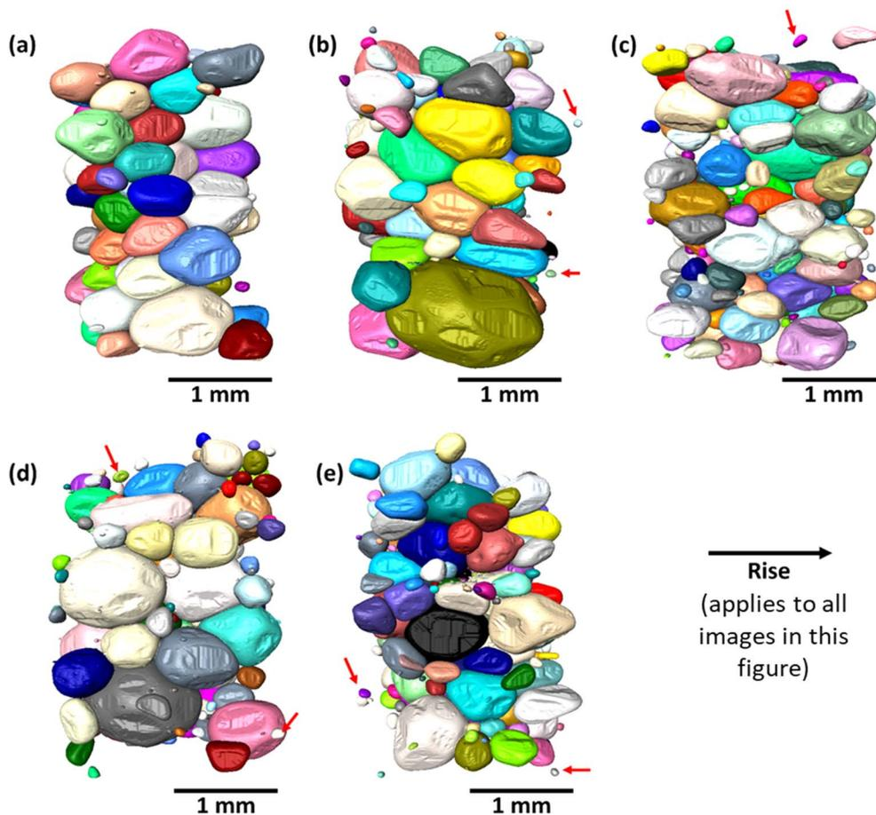
Fig. 2 3D renderings of separated pores within the foam structure generated from a mid-level resolution scan (pixel size  $3\ \mu\text{m}$ ). (a) Control sample, (b) 10FRH, (c) 30FRH, (d) 10CRH, (e) 30CRH. The black arrow indicates the direction of rising and red arrows point to examples of small, closed pores.
