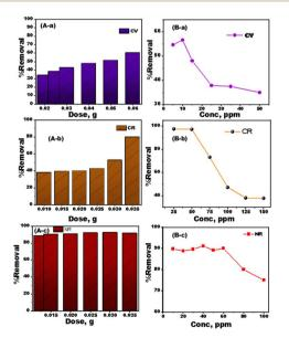
Fig. 4 (A) Effect of MDLZ nanocubes dosage on the adsorption capacity of the material for removal of (A-a) CV, (A-b) CR, and (A-c) NR dyes. (B) Effect of initial concentration of (B-a) CV, (B-b) CR, and (B-c) NR dyes at optimal conditions.
