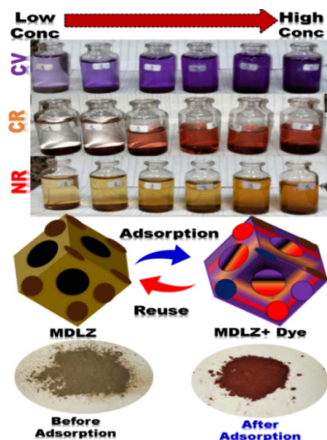
Scheme 1 The interactions between magnetite loaded and doped into cubic zinc metal–organic frameworks (MDLZ) adsorbent with CV, CR, and NR dye were examined at optimal conditions. The MDLZ adsorbent color changed from pale brown to reddish brown color, indicating the removal of the multiple dyes.
