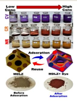
Scheme 1 The interactions between magnetite loaded and doped into cubic zinc metal-organic frameworks (MDLZ) adsorbent with CV, CR, and NR dye were examined at optimal conditions. The MDLZ adsorbent color changed from pale brown to reddish brown color, indicating the removal of the multiple dyes.
