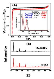
Fig. 2 (A)  $N_2$  adsorption/desorption isotherms and (inset) BJH pore size distribution of the ZN-MOF and MDLZ. (B) Wide-angle XRD diffraction patterns of the ZN-MOF and MDLZ nanocubes.
