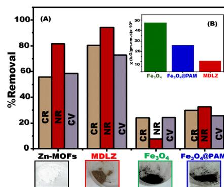
Fig. 8 (A) The comparison in removal percentage of CR, CV, and NR dyes using different adsorbents such as Zn-MOFs, MDLZ, Fe<sub>3</sub>O<sub>4</sub>, and Fe<sub>3</sub>O<sub>4</sub>@PAM under optimum adsorption conditions. (B) The magnetic susceptibility of MDLZ, Fe<sub>3</sub>O<sub>4</sub>, and Fe<sub>3</sub>O<sub>4</sub>@PAM.
