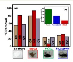
Fig. 8 (A) The comparison in removal percentage of CR, CV, and NR dyes using different adsorbents such as Zn-MOFs, MDLZ, Fe $_3$ O $_4$ , and Fe $_3$ O $_4$ @PAM under optimum adsorption conditions. (B) The magnetic susceptibility of MDLZ, Fe $_3$ O $_4$ , and Fe $_3$ O $_4$ @PAM.
