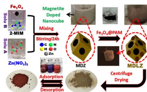
**Scheme 2** The preparation of magnetite loaded and doped with into cubic zinc metal–organic frameworks (MDLZ) adsorbent via mixing of zinc nitrate salt with magnetite and 2-methylimidazole as a linker. The brown precipitate of MDLZ was observed after mixing and stirring for 24 h. The brown powder were separated, cleaned, and dried. The obtained MDLZ nanocubes were utilized in removal of CV, CR, and NR dyes.
