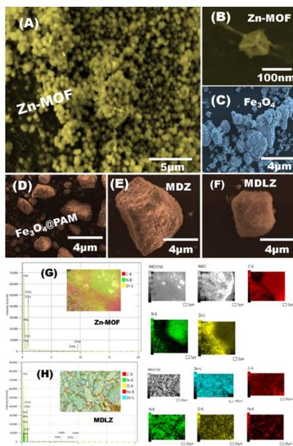
Fig. 1 Low- and high-magnification FESEM images of (A, B) the nanocube Zn-MOFs as intergrowing crystals, (C)  $\text{Fe}_3\text{O}_4$ , (D)  $\text{Fe}_3\text{O}_4$ @PAM, (E) MDZ and (F) cubic MDLZ adsorbent. FESEM-mapping of (G) Zn-MOFs and (H) MDLZ adsorbent.
