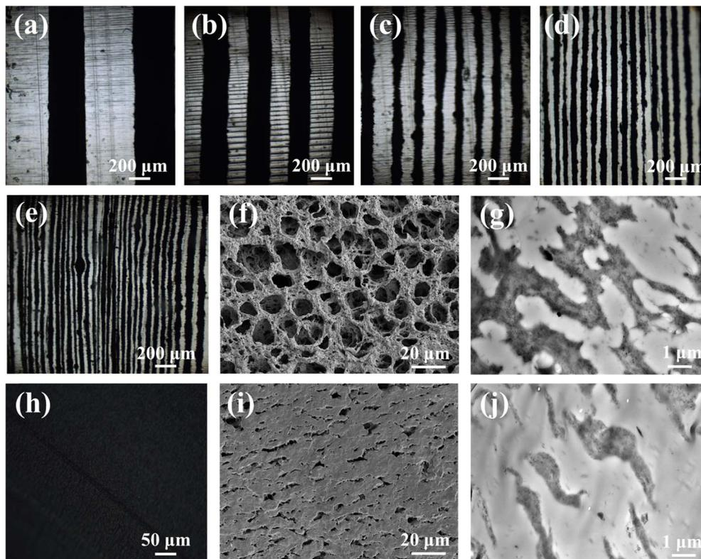
Fig. 2 (a–e) PLM images of the PLA/ALM multilayer composites; (f and g) SEM and TEM images of the individual ALM layer; and (h–j) PLM, SEM, and TEM images of CBC.
