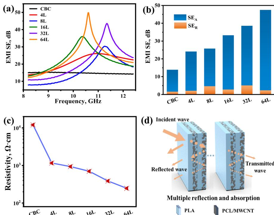
Fig. 5 (a) EMI SE of each composite in the X-Band. (b) SE<sub>A</sub> and SE<sub>R</sub>, and (c) electrical resistivity of each composite. (d) Schematic diagram of the EMI shielding mechanism of multilayer composites.
