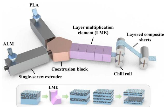
Fig. 1 Schematic of the layer-assembly coextrusion system.
