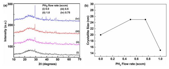
(a) XRD spectra of PH3 doped n type nc-Si:H films deposited at different PH3 flow rates (b) variation in crystallite size with PH3 flow rates.
