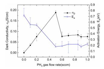
Fig. 8 Variation in dark conductivity  $(\sigma_D)$  and charge carrier activation energy  $(E_a)$  as a function of the PH<sub>3</sub> flow rates.
