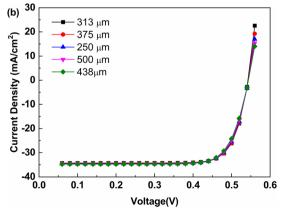
Fig. 10 Effect of thickness variation in (a) n type layer (b) p type layer on JV characteristics.
