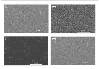
Fig. 3 Top view FESEM images of PH<sub>3</sub> doped n type nc-Si:H films grown at different PH<sub>3</sub> flow rates (a) 0.0 (b) 0.5 (c) 0.75 and (d) 1 sccm.
