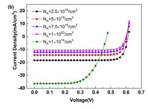
Fig. 19 Effect of doping in (a) n type layer (b) p type layer on JV characteristics.
