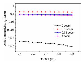
Fig. 7 Effect of temperature on dark conductivity ( $\sigma_D$ ) for different PH<sub>3</sub> flow rates.
