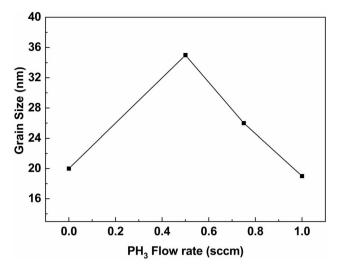
Fig. 4 Variation in the grain size due to increased PH<sub>3</sub> flow rates.
