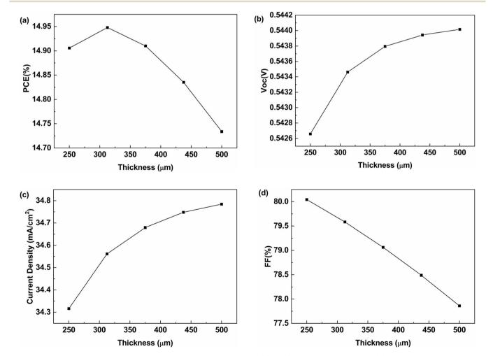
Fig. 13 Impact of thickness variation in p type layer on output parameters (a) PCE (b)  $V_{OC}$  (c) current density (d) FF.
