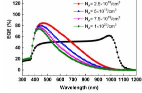
Fig. 18 Effect of doping in (a) n type layer (b) p type layer on EQE.
