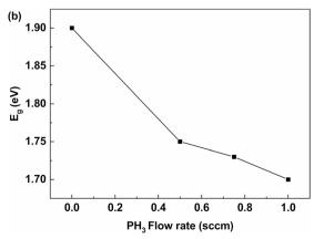
Fig. 5 (a) Tauc's plot of PH<sub>3</sub> doped films (b) change in optical band gap  $(E_n)$  with PH<sub>3</sub> flow rates.
