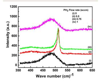
Fig. 1 Raman spectra of n type nc-Si:H films deposited at different  $\mathrm{PH}_3$  flow rates.
