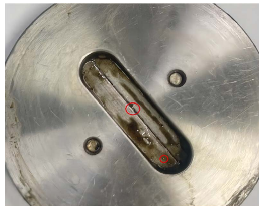
Fig. 10 The condition of the crack board in the plugging experiment of the crack width is 0.25\ \mu\text{m} .
