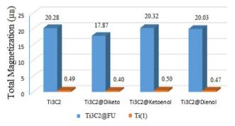
Fig. 6 Total magnetic moment of the  $Ti_1$  atom and  $Ti_3C_2$ @FU systems at the most stable adsorption sites.
