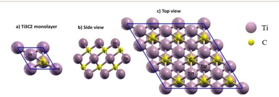
Fig. 1 (a)  $Ti_3C_2$  unit cell, (b) side and (c) top views of the  $3 \times 3 \times 1$  supercell of  $Ti_3C_2$  MXene. Three special sites for the absorption process are marked on the (c).
