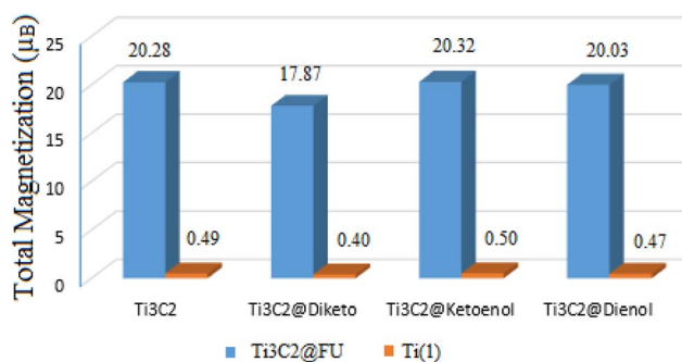
Fig. 6 Total magnetic moment of the \text{Ti}_1 atom and \text{Ti}_3\text{C}_2 @FU systems at the most stable adsorption sites.
