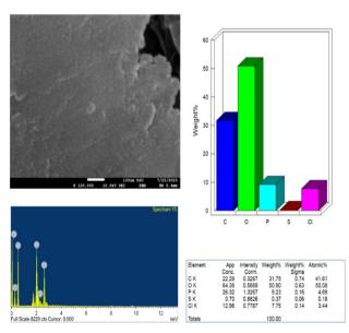
Fig. 10 EDX analysis of the synthesized PClCDs.
