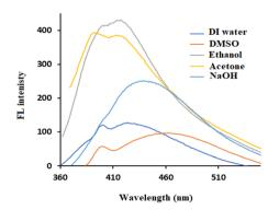
Fig. 1 FL spectra of lignin after hydrothermal treatment in different solvents at 200  $^{\circ}\text{C}$  for 12 h.
