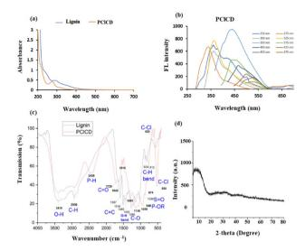
Fig. 8 (a) UV-vis absorption spectra of lignin and PClCDs, (b) FL spectra of PClCDs at different  $\lambda_{\rm ex}$  values, (c) FT-IR spectra of lignin and PClCDs, and (d) XRD spectrum of PClCDs.
