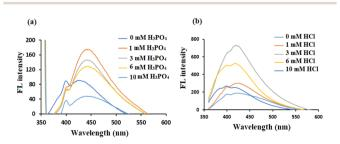
Fig. 5 FL spectra of modified lignin-based CDs with different amounts of dopant precursors (a)  $\rm H_3PO_4$  and (b) HCl.
