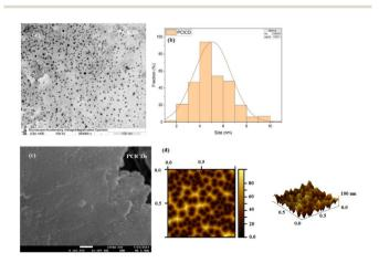
Fig. 7 (a) TEM image, (b) average particle size distribution using ImageJ software, (c) SEM image, and (d) AFM 3D image of PCICDs.
