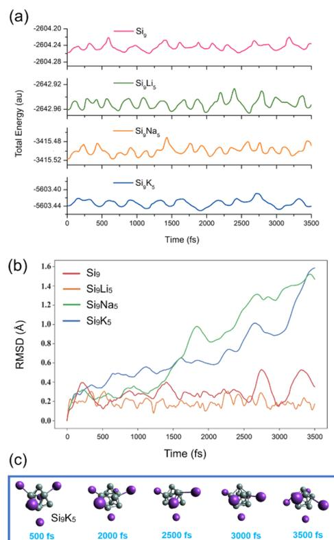
**Fig. 2** Time evolution of the (a) total energy, (b) root-mean-square deviation (RMSD), and (c) snapshots of the Si<sub>9</sub>K<sub>5</sub> geometries during *ab initio* molecular dynamics simulations at 300 K using the B3LYP-D3/def2-SVP method.
