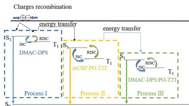
Fig. 3 Schematic diagram of energy transfer including RISC channels in EML of device A, B and C.
