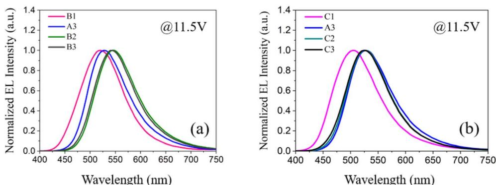
Fig. 5 (a) The normalized EL spectra of devices B1, A3, B2 and B3 at 11.5 V driving voltage; (b) the normalized EL spectra of devices C1, A3, C2 and C3 at 11.5 V driving voltage.
