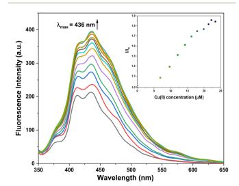
Fig. 6 Fluorescence titration of probe 3 with the successive addition of  $Cu^{2+}$  ions; inset exhibits the relative emission of 3 ( $I/I_o$ ) as a function of  $Cu^{2+}$  concentration ( $\mu$ M).
