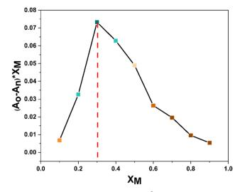
Fig. 7 Job plot analysis of probe 3 upon  $Cu^{2+}$  complexation indicating a 2:1 (L:M) stoichiometry.
