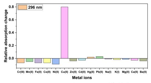
Relative absorption intensity changes of probe 3 on adding different metal ions in DMSO/H<sub>2</sub>O (4:1).
