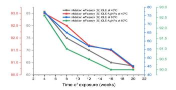
Fig. 7 Inhibition stability of the extracts
