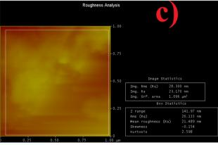
Fig. 8 AFM analysis of the corroded surface: (a) 0 g L $^{-1}$ , (b) 0.3 g L $^{-1}$  CLE, (c) 0.3 g L $^{-1}$  CLE-AgNPs.
