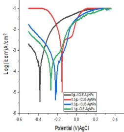
Fig. 5 Variation of the current density with the potential.
