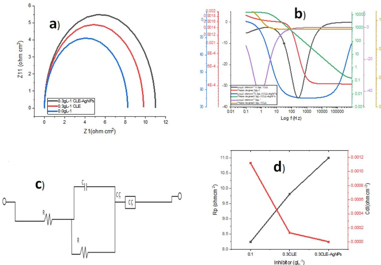
Fig. 6 (a) Nyquist curves and (b) Bode curve of the samples: 0 g L<sup>-1</sup>, 0.3 g L<sup>-1</sup> CLE and 0.3 g L<sup>-1</sup> CLE-AgNPs. (c) EIS fitting circuit model. (d) Plots of polarization resistance ( $R_p$ ) and capacitance of the interface ( $C_{dl}$ ) with inhibitor.
