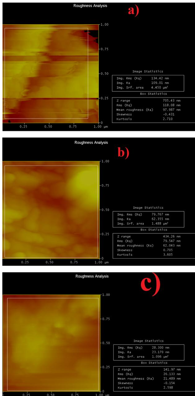
Fig. 8 AFM analysis of the corroded surface: (a) 0 g L<sup>-1</sup>, (b) 0.3 g L<sup>-1</sup> CLE, (c) 0.3 g L<sup>-1</sup> CLE-AgNPs.
