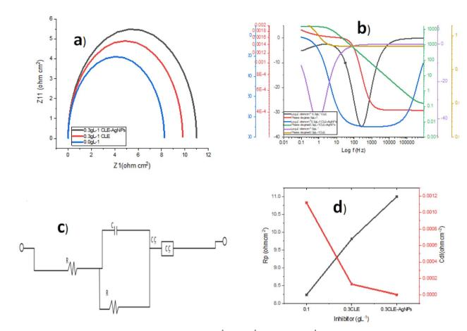
Fig. 6 (a) Nyquist curves and (b) Bode curve of the samples:  $0 \text{ g L}^{-1}$ ,  $0.3 \text{ g L}^{-1}$  CLE and  $0.3 \text{ g L}^{-1}$  CLE-AgNPs. (c) EIS fitting circuit model. (d) Plots of polarization resistance ( $R_p$ ) and capacitance of the interface ( $C_{dl}$ ) with inhibitor.
