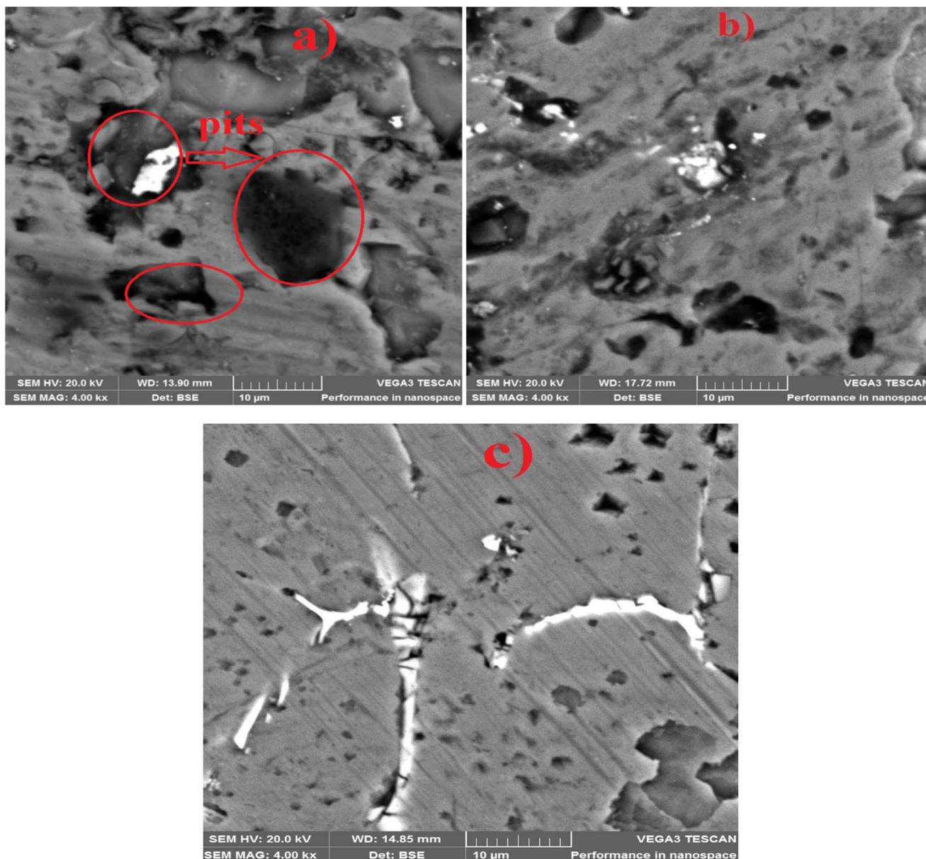
Fig. 9 Corroded surfaces of (a)  $0 \text{ g L}^{-1}$ , (b)  $0.3 \text{ g L}^{-1}$  CLE, (c)  $0.3 \text{ g L}^{-1}$  CLE-AgNPs.
