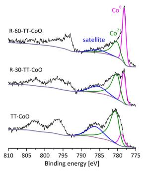
Fig. 2 XPS Co 2p spectra of TT-CoO, R-30-TT-CoO, and R-60-CoO thin-film catalysts.
