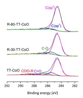
Fig. 3  $\,$  XPS C 1s spectra of TT-CoO, R-30-TT-CoO, and R-60-TT-CoO thin-film catalysts.
