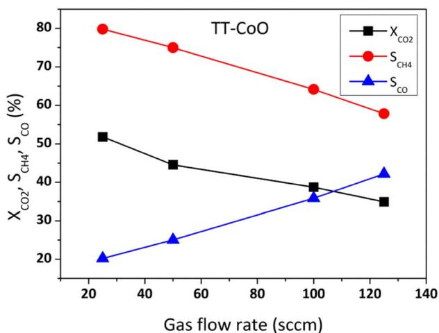
Fig. 5 CO<sub>2</sub> hydrogenation performance of TT-CoO catalyst at different gas flow rates at 400 °C. Reaction conditions:  $P = 0.1$  MPa,  $\text{H}_2/\text{CO}_2 = 4$ .
