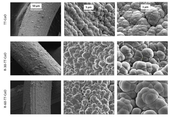
Fig. 1 SEM morphology of TT-CoO, R-30-TT-CoO, and R-60-TT-CoO thin-film catalysts.
