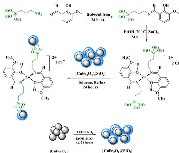
Scheme 2 The preparation of nano- $[\text{CuFe}_2\text{O}_4@/\text{SiO}_2/\text{propyl-1-(O-vanillinaldimine)}][\text{ZnCl}_2]$ .
