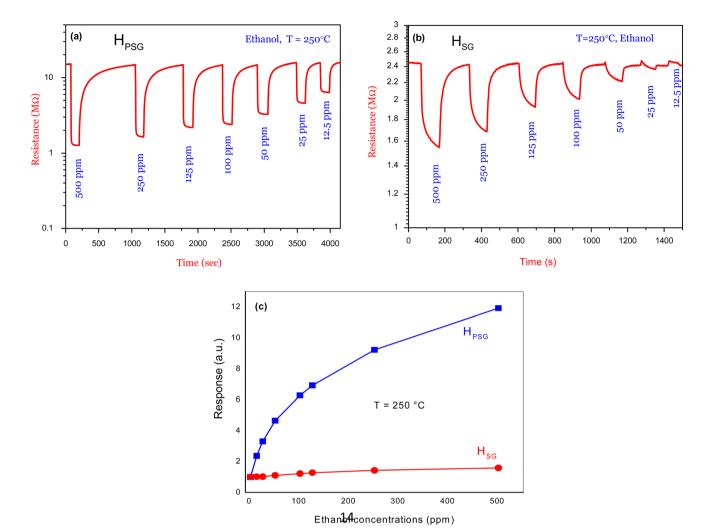
Fig. 6 Dynamic resistance curves of (a)  $H_{SG}$  sensor and (b)  $H_{PSG}$  sensor to various concentrations of ethanol at 250 °C (c) corresponding calibration curves.
