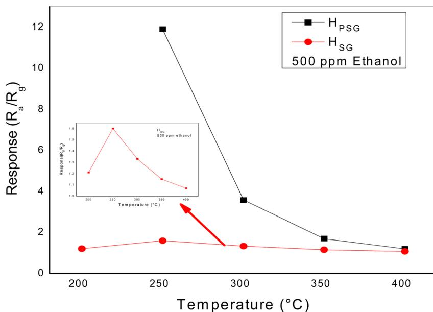
Fig. 5 Gas response versus the working temperature of the  $\alpha$ - $Fe_2O_3$  sensors.
