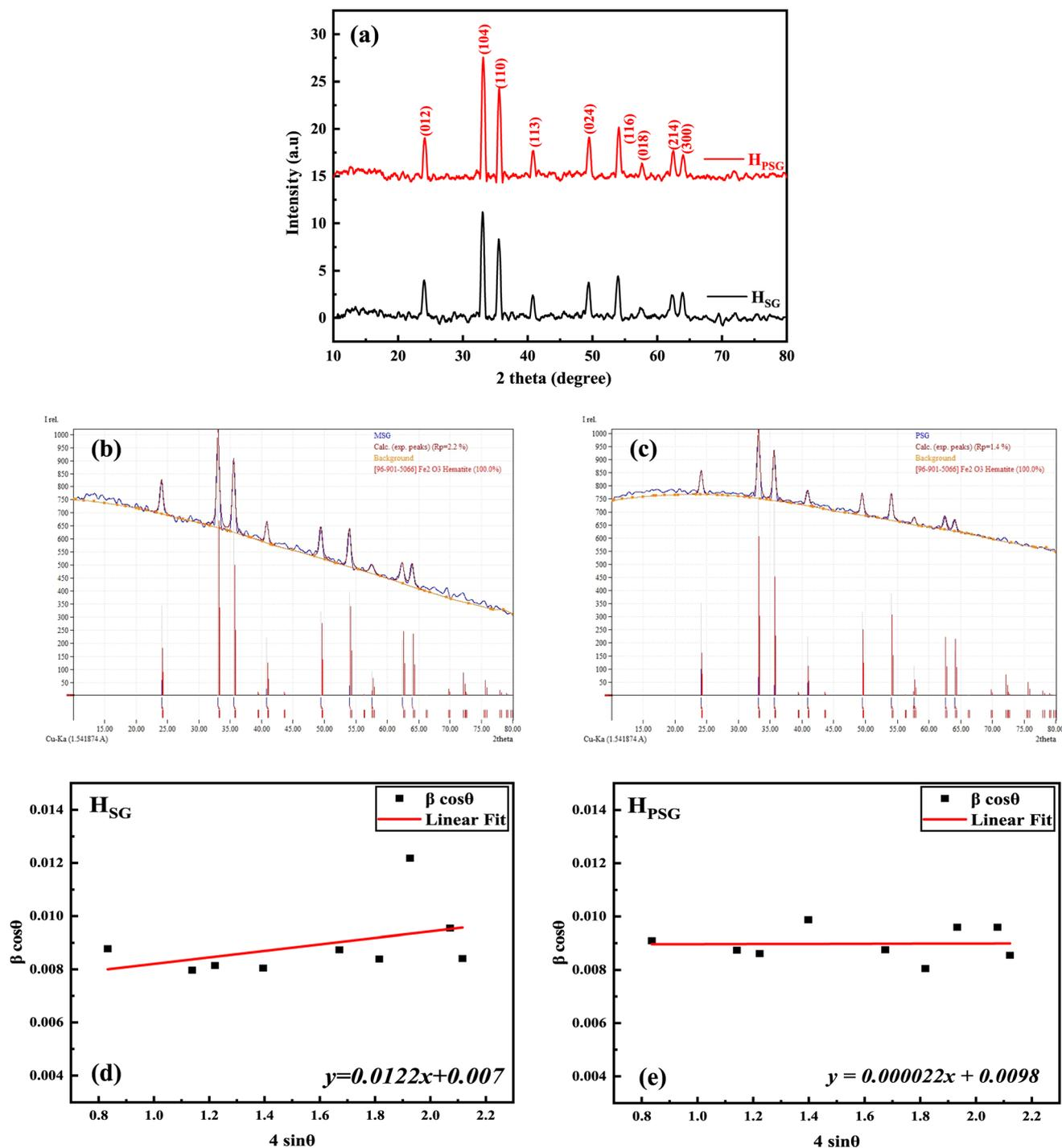
Fig. 2 (a) XRD pattern of H<sub>PSG</sub> and H<sub>SG</sub> samples. (b) The Rietveld refinement plot of the H<sub>PSG</sub> sample. (c) The Rietveld refinement plot of the H<sub>SG</sub> sample (the blue curve represents the observed data and the oily color is the calculated pattern; the light blue curve shows the difference between the observed and calculated intensities). (d) Williamson–Hall plots of the H<sub>PSG</sub> sample. (e) Williamson–Hall plots of the H<sub>SG</sub> sample.
