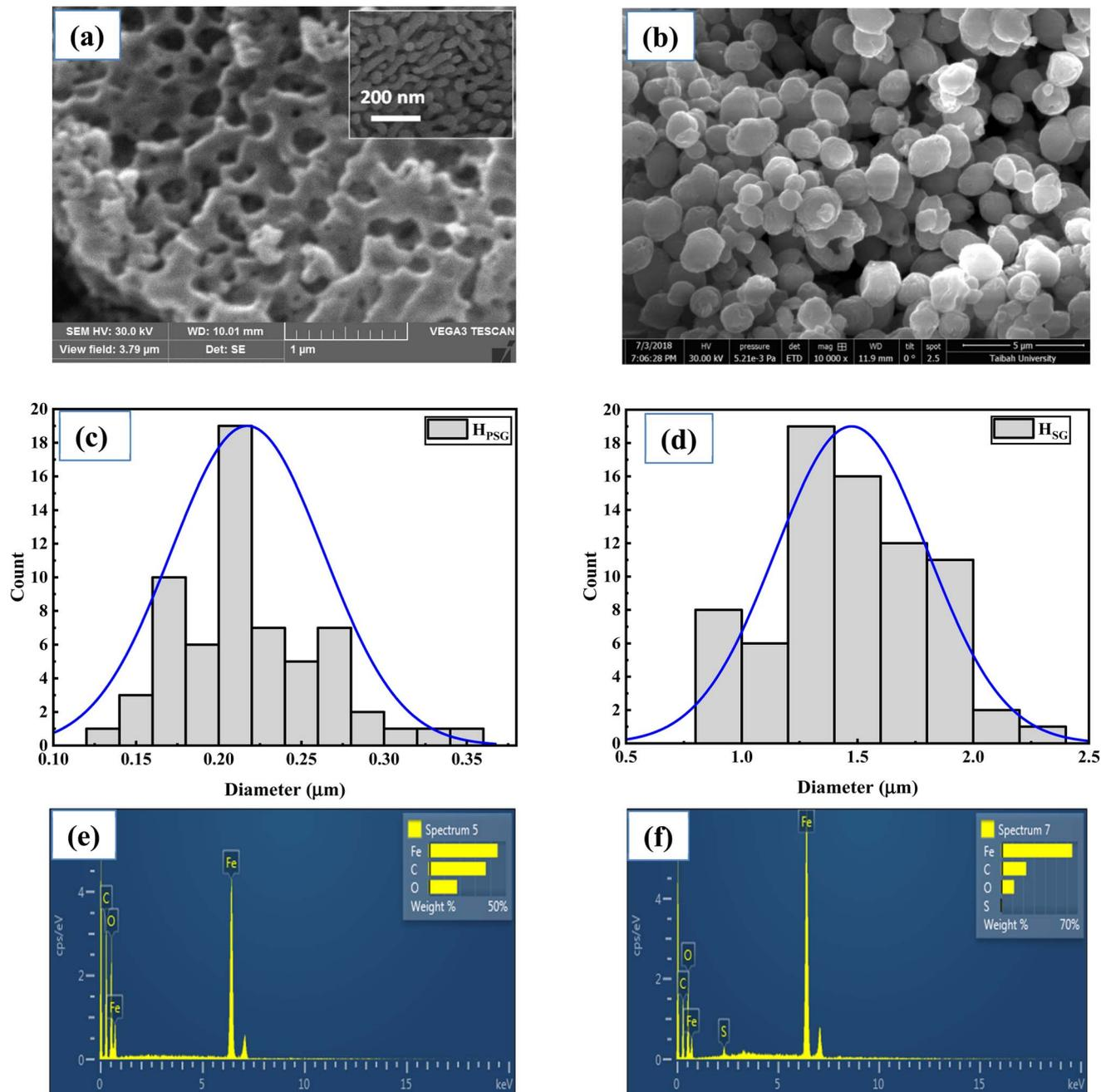
Fig. 3 SEM images of the (a) H<sub>PSG</sub> and (b) H<sub>SG</sub> samples. Inset in (a) shows higher magnification image. Particles size distribution of the (c) H<sub>PSG</sub> and (d) H<sub>SG</sub> samples. EDS spectra of the (e) H<sub>PSG</sub> and (f) H<sub>SG</sub> samples.
