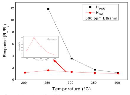
Fig. 5 Gas response versus the working temperature of the  $\alpha$ -Fe<sub>2</sub>O<sub>3</sub> sensors.
