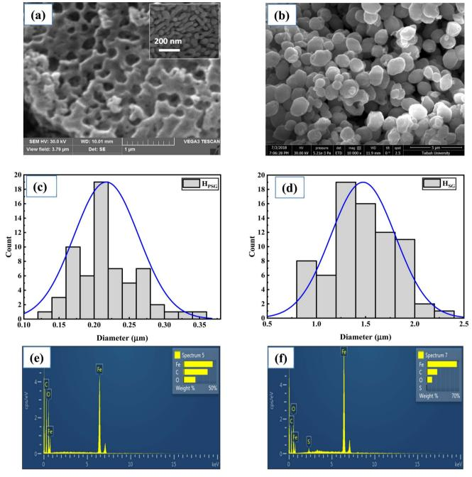
Fig. 3 SEM images of the (a)  $H_{PSG}$  and (b)  $H_{SG}$  samples. Inset in (a) shows higher magnification image. Particles size distribution of the (c)  $H_{PSG}$  and (d)  $H_{SG}$  samples. EDS spectra of the (e)  $H_{PSG}$  and (f)  $H_{SG}$  samples.
