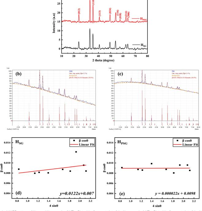
Fig. 2 (a) XRD pattern of  $H_{PSG}$  and  $H_{SG}$  samples. (b) The Rietveld refinement plot of the  $H_{PSG}$  sample. (c) The Rietveld refinement plot of the  $H_{SG}$  sample (the blue curve represents the observed data and the oily color is the calculated pattern; the light blue curve shows the difference between the observed and calculated intensities). (d) Williamson–Hall plots of the  $H_{PSG}$  sample. (e) Williamson–Hall plots of the  $H_{SG}$  sample.
