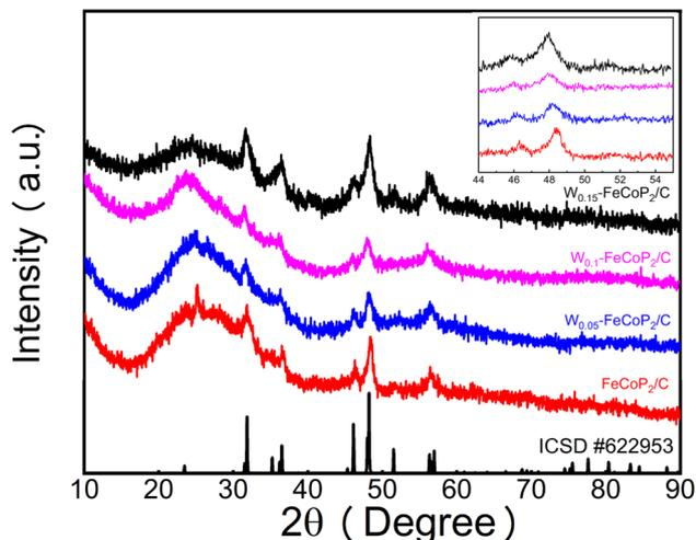
Fig. 1 XRD patterns of the  $W_{0.1}$ -FeCoP<sub>2</sub>/C,  $W_{0.15}$ -FeCoP<sub>2</sub>/C,  $W_{0.05}$ -FeCoP<sub>2</sub>/C and FeCoP<sub>2</sub>/C.
