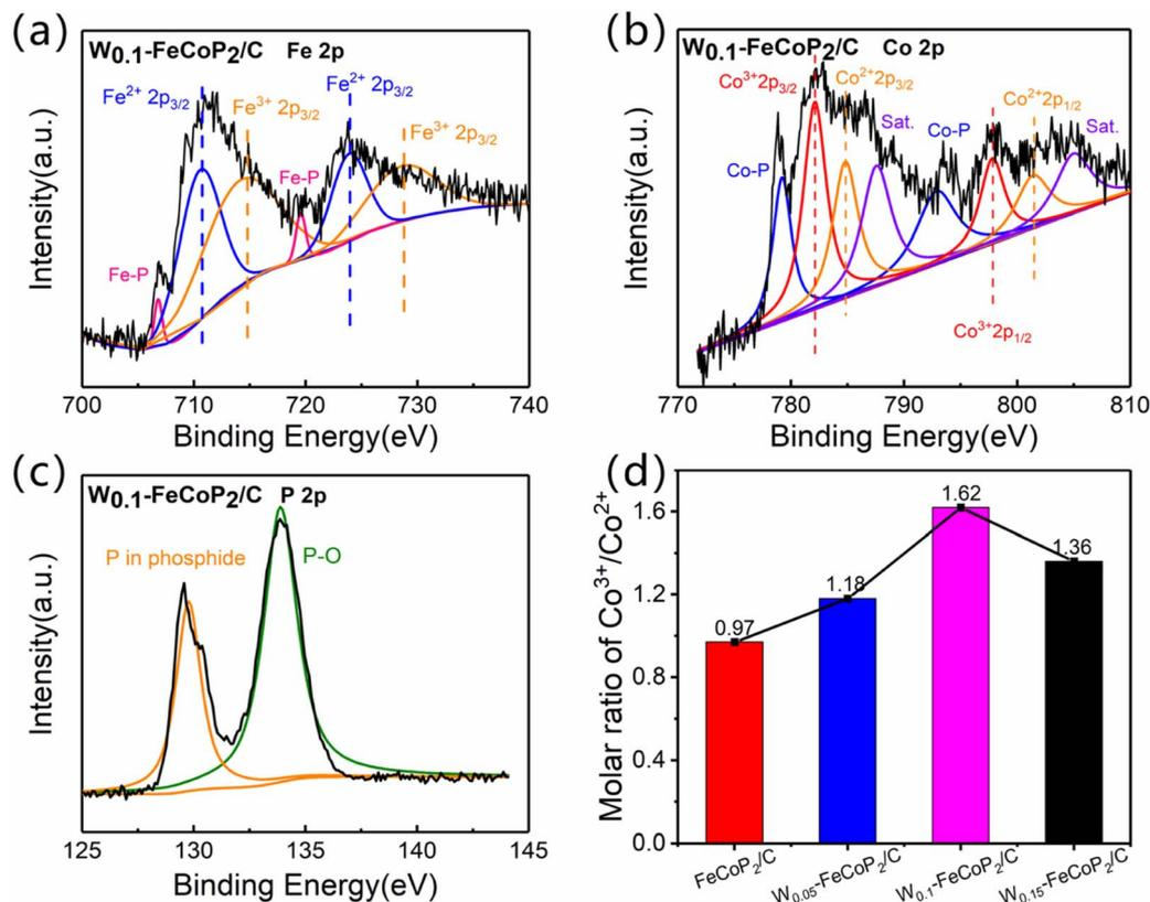
Fig. 3 (a) Fe 2p XPS spectra for W<sub>0.1</sub>-FeCoP<sub>2</sub>/C; (b) Co 2p XPS spectra for W<sub>0.1</sub>-FeCoP<sub>2</sub>/C; (c) P 2p XPS spectra for W<sub>0.1</sub>-FeCoP<sub>2</sub>/C; (d) Co<sup>3+</sup>/Co<sup>2+</sup> molar ratios of FeCoP<sub>2</sub>/C, W<sub>0.05</sub>-FeCoP<sub>2</sub>/C, W<sub>0.1</sub>-FeCoP<sub>2</sub>/C and W<sub>0.15</sub>-FeCoP<sub>2</sub>/C.
