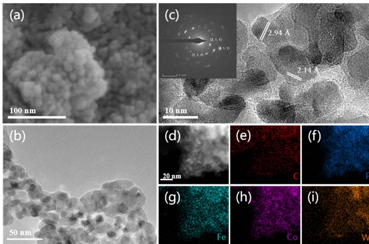
Fig. 2 (a) SEM image of  $W_{0.1}$ -FeCoP<sub>2</sub>/C in different magnification (b) TEM image of  $W_{0.1}$ -FeCoP<sub>2</sub>/C (c) high-resolution TEM image of the  $W_{0.1}$ -FeCoP<sub>2</sub>/C nanostructure with a corresponding fast Fourier transform pattern (d) HADDF-TEM image of the  $W_{0.1}$ -FeCoP<sub>2</sub>/C and the corresponding elemental mapping of (e) carbon (f) phosphorus (g) cobalt (h) iron and (i) tungsten.
