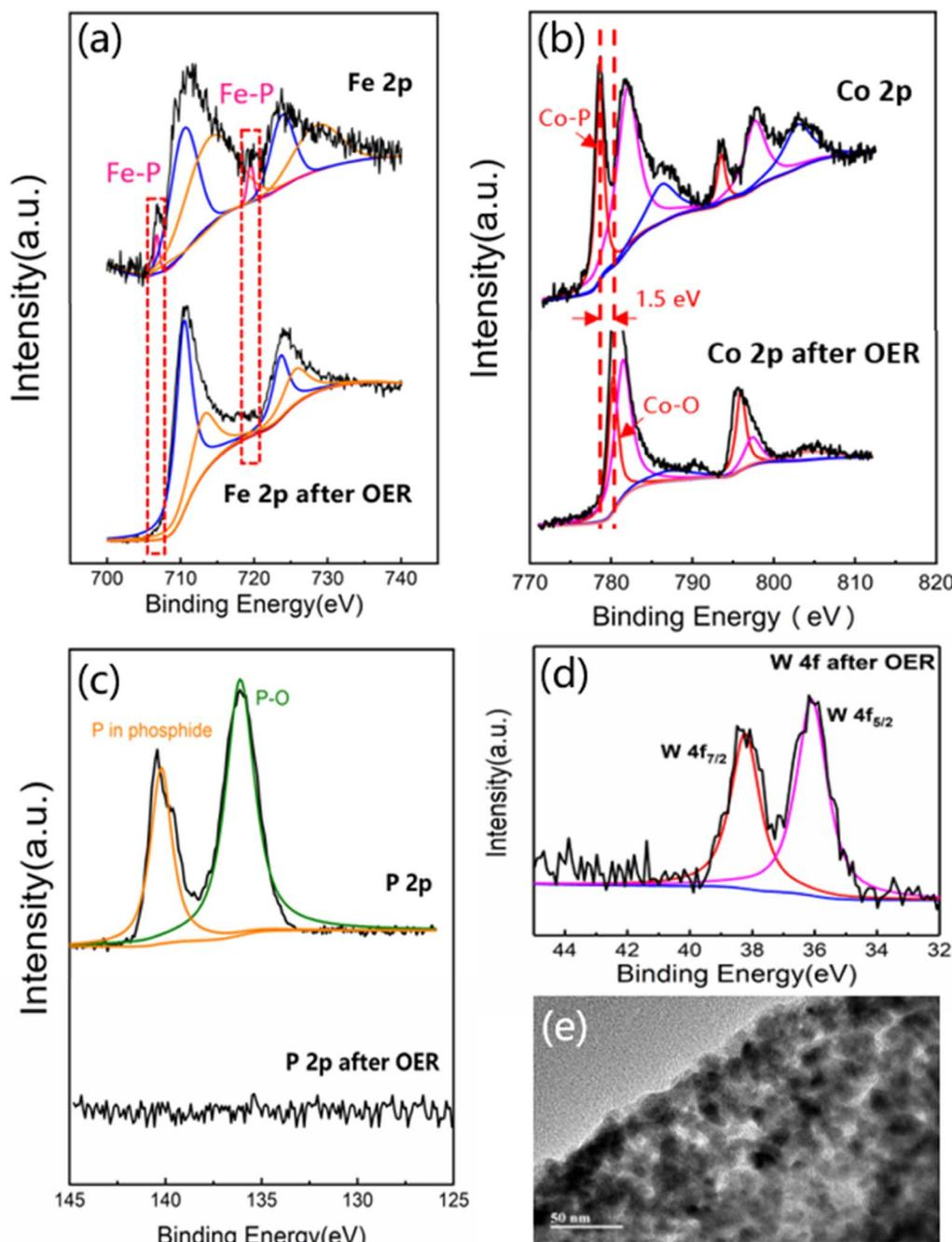
Fig. 5 The comparison of the high-resolution XPS spectra of  $W_{0.1}$ -FeCoP<sub>2</sub>/C before (top) and after (bottom) OER tests: (a) Fe 2p, (b) Co 2p, and (c) P 2p; (d) XPS characterization of W 4f and (e) TEM image of  $W_{0.1}$ -FeCoP<sub>2</sub>/C after OER tests.
