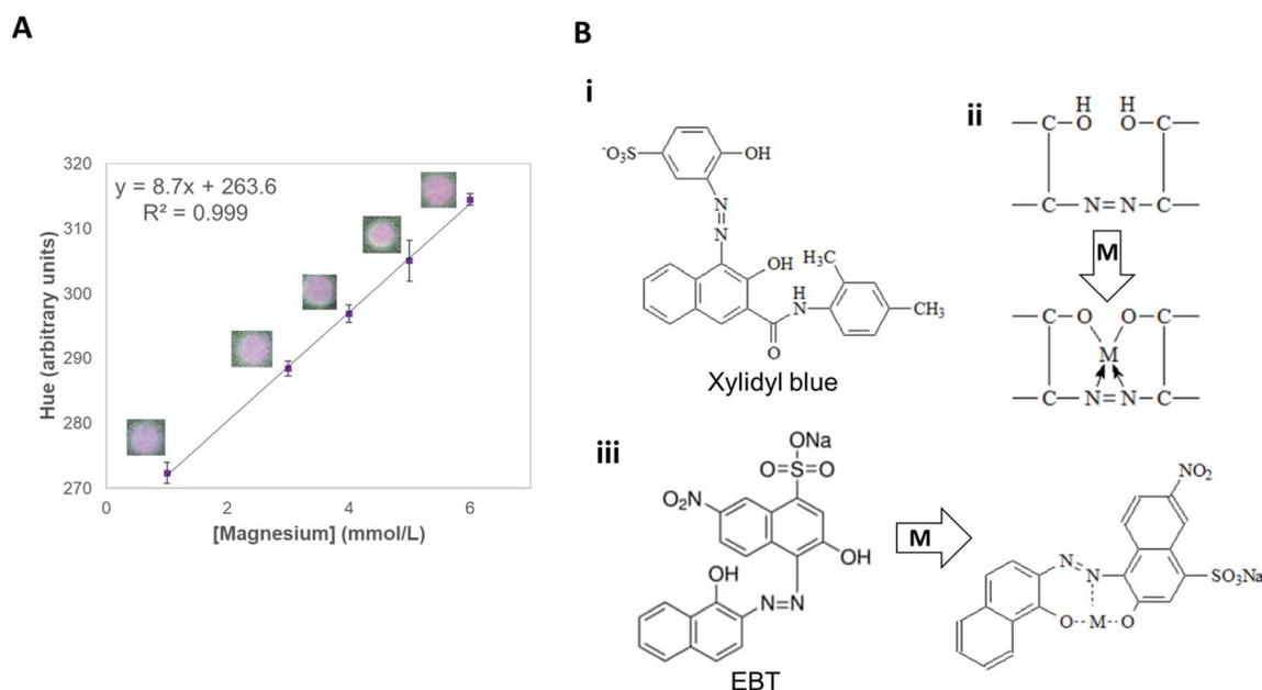
Fig. 4 Detection of magnesium in the proposed  $\mu$ PAD. (A) Calibration curve obtained for  $\text{Mg}^{2+}$  in concentrations ranging from 1.0 to 6.0  $\text{mmol L}^{-1}$ . (B) Structure of (i) Xylydyl blue before the interaction with the analyte; (ii) the region of Xylydyl blue responsible for binding to  $\text{Mg}^{2+}$  before and after the interaction; and (iii) EBT before and after binding to  $\text{Mg}^{2+}$ .
