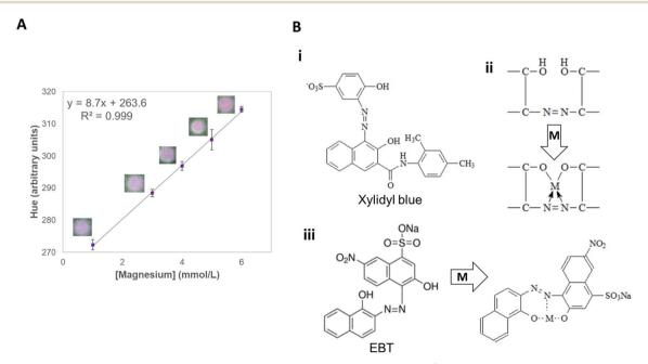
Fig. 4 Detection of magnesium in the proposed  $\mu$ PAD. (A) Calibration curve obtained for Mg<sup>2+</sup> in concentrations ranging from 1.0 to 6.0 mmol L<sup>-1</sup>. (B) Structure of (i) Xylidyl blue before the interaction with the analyte; (ii) the region of Xylidyl blue responsible for binding to Mg<sup>2+</sup> before and after the interaction; and (iii) EBT before and after binding to Mg<sup>2+</sup>.
