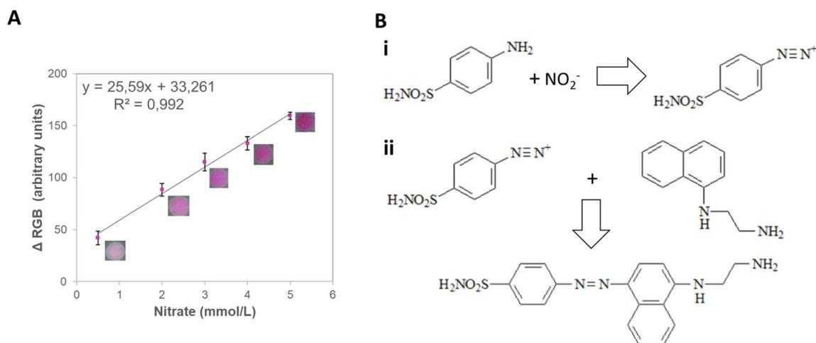
Fig. 6 Detection of nitrate in the proposed  $\mu\text{PAD}$ . (A) Calibration curve obtained for ammonium in concentrations ranging from 0.5 to 10.0  $\text{mmol L}^{-1}$ . (B) Reaction between (i) nitrite and sulfanilamide, forming a diazo compound; (ii) diazo compound and NED, forming an azo dye with a red-purple color, allowing the quantification of nitrate.
