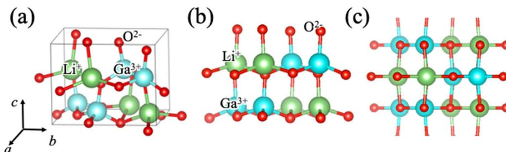
Fig. 1 (a) Schematic illustration of LiGaO<sub>2</sub> crystal structure. (b) The initial state of polarization switching and (c) the intermediate state of polarization switching in LiGaO<sub>2</sub>.
