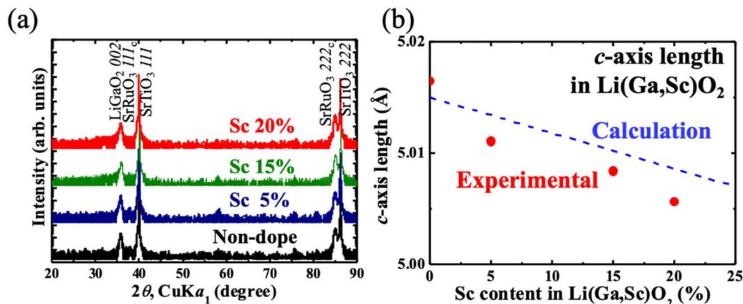
Fig. 3 (a) Out-of-plane XRD profiles of  $\text{LiGa}_{1-x}\text{Sc}_x\text{O}_2/(111)\text{SrTiO}_3$  ( $x = 0, 0.05, 0.15, 0.20$ ). (b) The  $c$ -axis lengths of prepared thin films with calculated values (blue dashed line).
