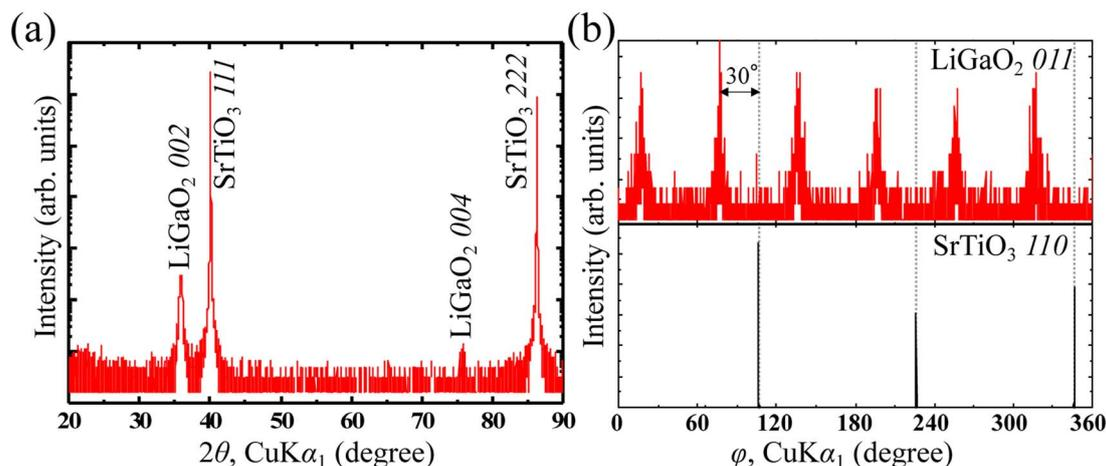
Fig. 2 (a) Out-of-plane XRD profiles of LiGaO<sub>2</sub>/(111)SrTiO<sub>3</sub>. (b) Phi-scan XRD patterns of LiGaO<sub>2</sub> 011 and SrTiO<sub>3</sub> 110.
