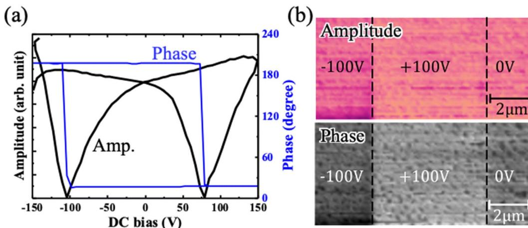
Fig. 4 (a) PFM results of amplitude (black line) and phase (blue line) signals in  $\text{LiGa}_{0.8}\text{Sc}_{0.2}\text{O}_2/\text{SrRuO}_3/(111)\text{SrTiO}_3$ . (b) PFM images of amplitude and phase for written sample in  $\text{LiGa}_{0.8}\text{Sc}_{0.2}\text{O}_2/\text{SrRuO}_3/(111)\text{SrTiO}_3$ .
