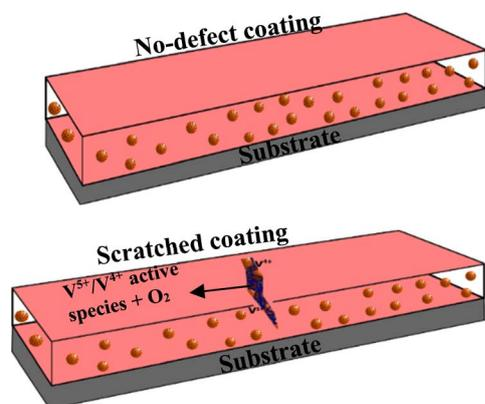
Fig. 10 Schematic of the proposed self-healing mechanism of artificially scratched epoxy coating embedding CS-ZrV microcapsules.
