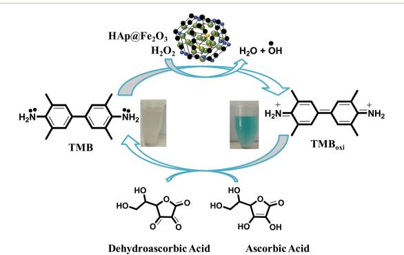
Scheme 1 Proposed mechanism for the sensing of ascorbic acid based on the HAp@Fe<sub>2</sub>O<sub>3</sub> mimic enzyme assisted by H<sub>2</sub>O<sub>2</sub>.
