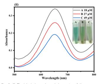
Fig. 6 (i) Physiological sample analysis spectra of the proposed sensor. Different concentrations of ascorbic acid in physiological solution at optimized conditions [4 mg HAp@Fe $_2O_3$ , 150  $\mu$ L TMB (12 mM), 100  $\mu$ L (24 mM) hydrogen peroxide, and 120  $\mu$ L ascorbic acid (56  $\mu$ M)]. (ii) shows the colorimetric response of the proposed sensor and the corresponding UV-Vis spectra under optimized conditions for the sensing of ascorbic acid in real samples.
