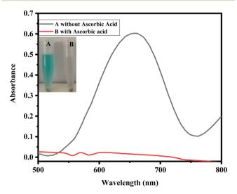
Fig. 2 UV-Vis spectra of the sensing reaction. The addition of 4 mg HAp@Fe $_2$ O $_3$ , 150  $\mu$ L TMB (12 mM), 100  $\mu$ L (24 mM) hydrogen peroxide, and 120  $\mu$ L (A) without ascorbic acid and (B) with 150  $\mu$ L ascorbic acid (56  $\mu$ M).
