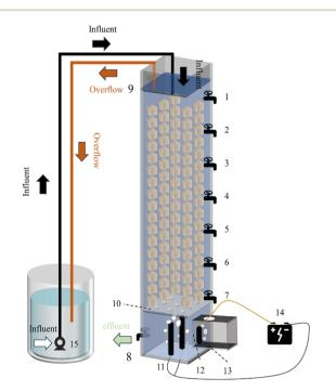
Fig. 1 1–8: sample port; 9: overflow port; 10: perforated partition; 11: cathode; 12: proton exchange membrane; 13: anode; 14: power supply; 15: pump.
