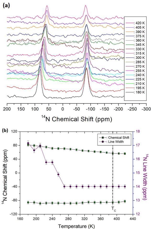
Fig. 6 (a). Static NMR spectrum for  $^{14}\text{N}$  in  $\text{N}(\text{CH}_3)_4\text{CdBr}_3$  single crystal as the temperature rises. (b). Static NMR chemical shifts and line widths for  $^{14}\text{N}$  in  $\text{N}(\text{CH}_3)_4\text{CdBr}_3$  single crystal as the temperature rises.
