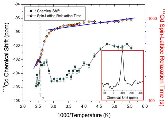
Fig. 7 Static NMR chemical shifts and spin–lattice relaxation times in the laboratory system  $T_1$  for  $^{113}\text{Cd}$  in  $\text{N}(\text{CH}_3)_4\text{CdBr}_3$  single crystal as a function of inverse temperature. The slopes of the solid lines are represented activation energies ((Inset): The  $^{113}\text{Cd}$  NMR spectrum at 200 K).
