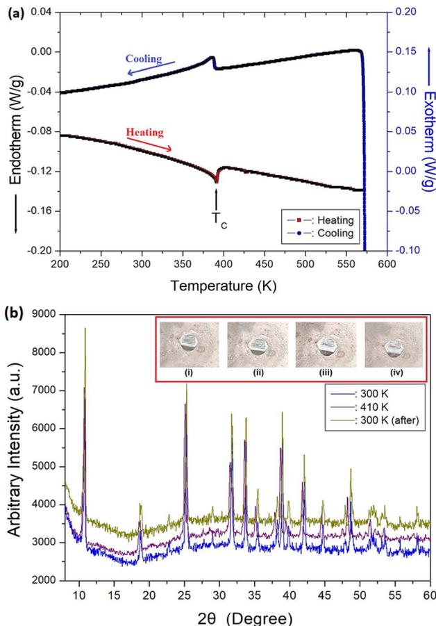
Fig. 2 (a). Differential scanning calorimetry curves at heating and cooling rate of  $10 \text{ }^\circ\text{C min}^{-1}$ . (b). The powder X-ray diffraction patterns at 300, 410, and 300 K (after) ((Inset): the morphologies at (i) 300 K, (ii) 350 K, (iii) 430 K, and (iv) 300 K (after cooling) of  $N(\text{CH}_3)_4\text{CdBr}_3$  single crystal).
