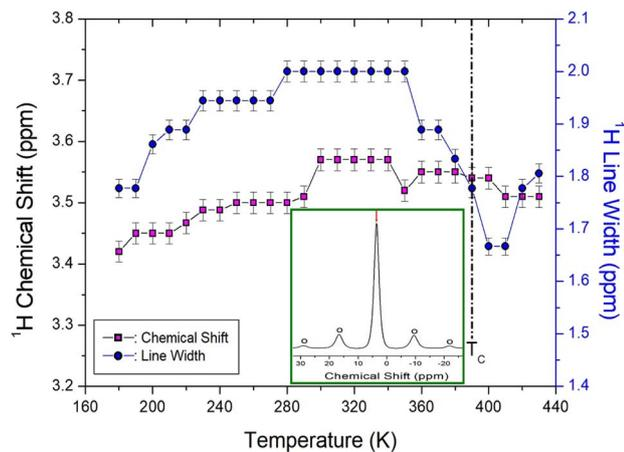
Fig. 3 NMR chemical shifts and line widths for  $^1\text{H}$  in  $\text{N}(\text{CH}_3)_4\text{CdBr}_3$  as the temperature rises ((Inset): The  $^1\text{H}$  NMR spectrum at 300 K, and open circles are spinning sidebands).
