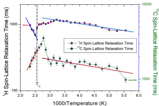
Fig. 5 The spin-lattice relaxation times in the rotating system  $T_{1\rho}$  for  $^1\text{H}$  and  $^{13}\text{C}$  in  $\text{N}(\text{CH}_3)_4\text{CdBr}_3$  as a function of inverse temperature. The slopes of the solid lines are represented activation energies.
