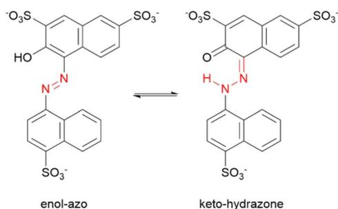
Scheme 1 Equilibrium of enol-azo (N=N) and keto-hydrazone (C=N-N-H) tautomeric forms for azo dye AMA. Azo and hydrazone groups are highlighted in red.
