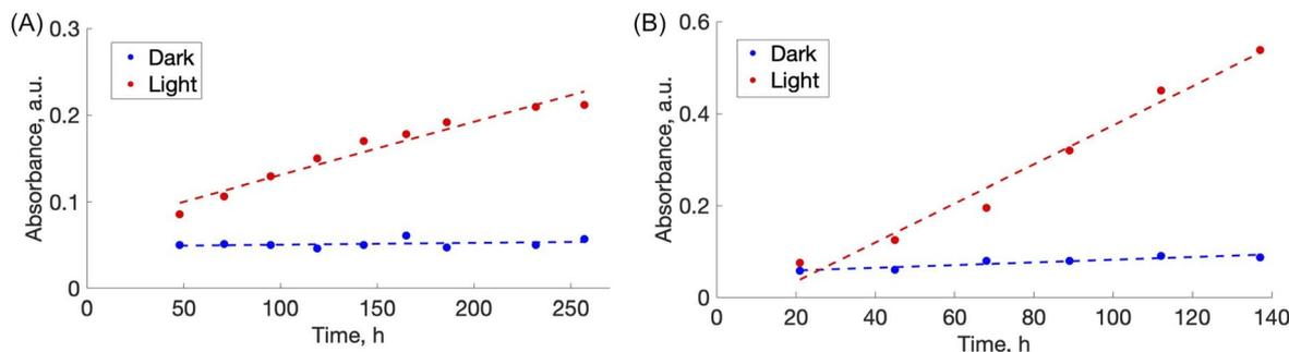
Fig. 5 (A) Change with time of the absorbance maxima of AMA in aqueous solution during disassembly of the free-standing thick film CS-AMA. The trendline equations for "absorbance – time" fit is  $A = 0.0007t + 0.0616$  for light and  $A = 6 \times 10^{-6}t + 0.0499$  for dark. (B) Change with time of the absorbance maxima of ALR in solution during disassembly of the free-standing thick film CS-ALR.
