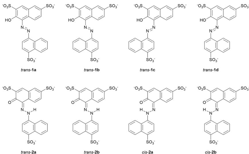
Chart 1 Possible conformers and isomeric forms of enol-azo AMA (**1**) and keto-hydrazone AMA (**2**) investigated at the B3LYP-D3BJ/ma-def2-TZVP level. Structures for *cis*-**1** have been omitted for simplicity.
