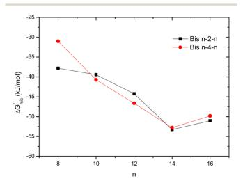
**Fig. 7** Variation of Gibbs energy of micellization of gemini surfactants with the length of the hydrophobic chain.
