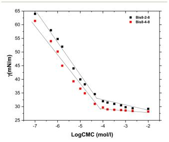
Fig. 1 Equilibrium surface tension ( $\gamma$ ) versus the logarithm of Bis 8-s-8 surfactant concentration curves.
