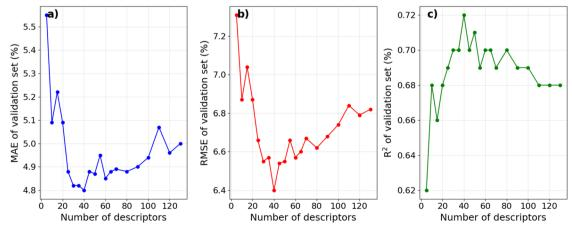
Fig. 2 Average MAE, RMSE, and R<sup>2</sup> of the validation sets in the 10-fold CV depend on the number of selected top descriptors.
