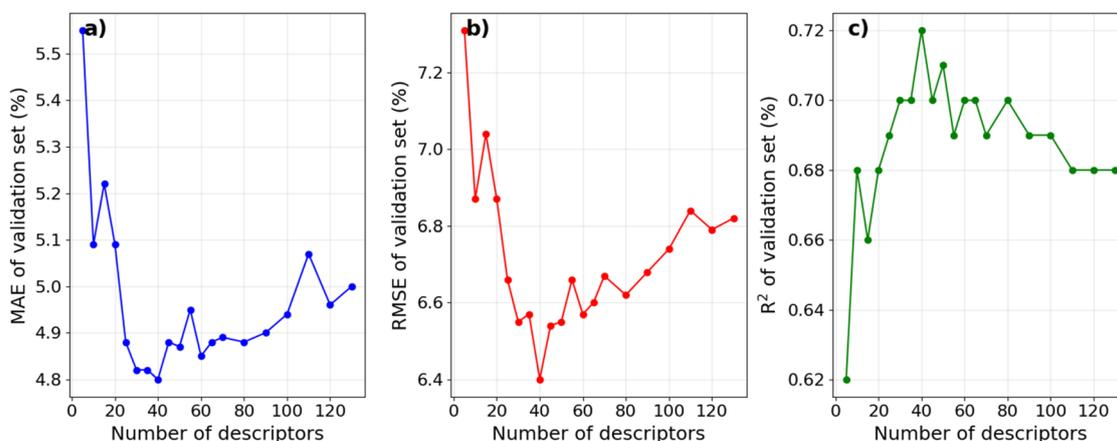
Fig. 2 Average MAE, RMSE, and  $R^2$  of the validation sets in the 10-fold CV depend on the number of selected top descriptors.
