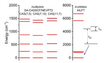
Fig. 5 The energies of six lowest multiplets as obtained from SA-CASSCF/NEVPT2 calculations using isolated  $[CoCl_4(C_5H_7N_3)_2]^{2-}$  anion for different CAS including the energies of d-orbitals obtained from AILFT analysis in the case of CAS(7,5).
