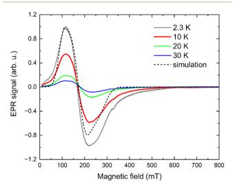
Fig. 6 X-band EPR spectra of I measured at 2, 10, 20 and 30 K (solid lines) including a simulation (dashed line) using an effective  $S_{\rm eff} = 1/2$ model.
