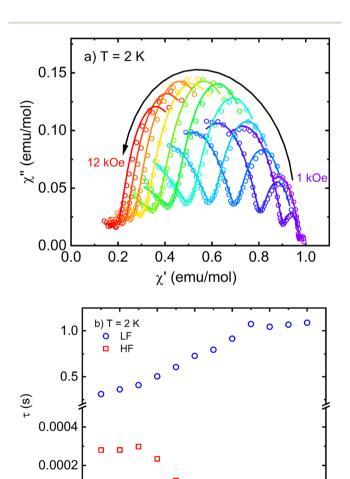
Fig. 7 (a) Cole-Cole plots of I in different applied DC fields measured at 2 K including the fits of the modified Debye model with two relaxation channels. (b) Field dependence of relaxation times extracted from Cole-Cole plots
