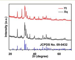
Fig. 2 XRD pattern of Xg-HAP and Yt-HAP.
