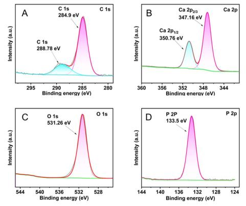
Fig. 13 XPS spectra of the Xq-HAP after fluoride adsorption: (A) C 1s, (B) Ca 2p, (C) O 1s, and (C) P 2p.
