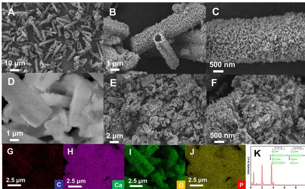
Fig. 3 (A–D) Xq-HAP SEM images, (E and F) Yt-HAP SEM images, (G–J) EDS elemental mapping for C, Ca, O and P respectively. (K) EDS spectrum of Xq-HAP.
