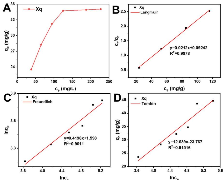
Fig. 10 (A) Adsorption isotherms of fluoride on Xq-HAP samples (dosage = 1 g L<sup>-1</sup>, T = 25 °C, contact time = 24 h, and pH = 7), (B) Langmuir isotherm model, (C) Freundlich isotherm model, and (D) Temkin isotherm model.
