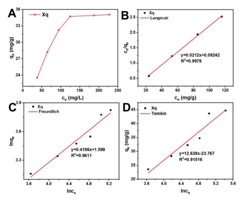
Fig. 10 (A) Adsorption isotherms of fluoride on Xq-HAP samples (dosage = 1 g  $L^{-1}$ , T = 25 °C, contact time = 24 h, and pH = 7), (B) Langmuir isotherm model, (C) Freundlich isotherm model, and (D) Temkin isotherm model
