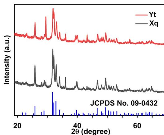
Fig. 2 XRD pattern of Xq-HAP and Yt-HAP.
