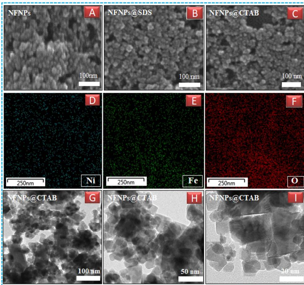
Fig. 3 Scanning electron microscope images of (A)  $\text{NiFe}_2\text{O}_4$  (B)  $\text{NiFe}_2\text{O}_4@\text{SDS}$  (C)  $\text{NiFe}_2\text{O}_4@\text{CTAB}$ , Elemental mapping micrographs (D) nickel-K $\alpha$  (E) iron-K $\alpha$  (F) oxygen-K $\alpha$ , Transmission electron microscope images of  $\text{NiFe}_2\text{O}_4@\text{CTAB}$  at (G) 100 nm (H) 50 nm, and (I) 20 nm.
