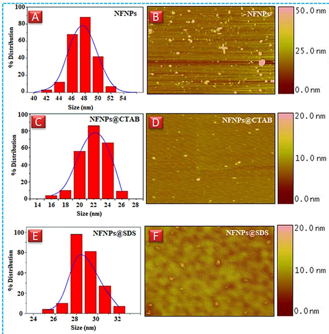
Fig. 2 Dynamic light scattering images of (A)  $\text{NiFe}_2\text{O}_4$  (C)  $\text{NiFe}_2\text{O}_4$ @CTAB (E)  $\text{NiFe}_2\text{O}_4$ @SDS, atomic force microscopy images (B)  $\text{NiFe}_2\text{O}_4$  (D)  $\text{NiFe}_2\text{O}_4$ @CTAB, and (F)  $\text{NiFe}_2\text{O}_4$ @SDS.
