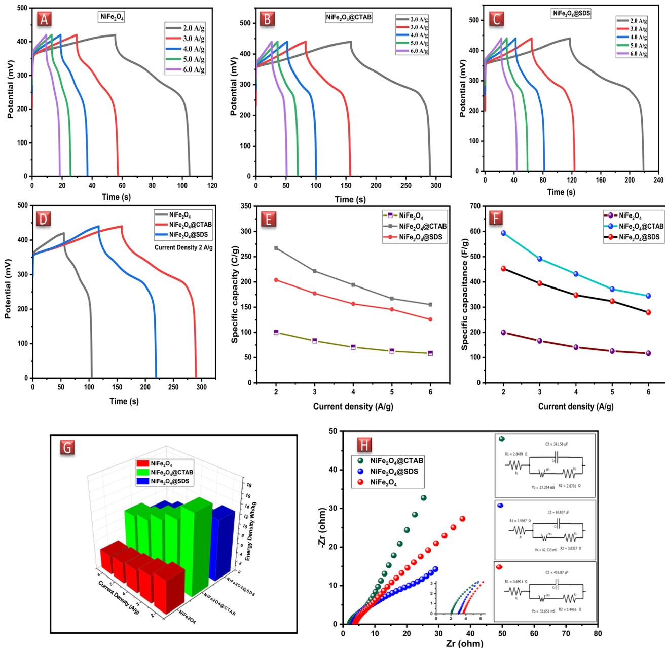
Fig. 5 (A) GCD measurements of  $\text{NiFe}_2\text{O}_4$ , (B)  $\text{NiFe}_2\text{O}_4@\text{CTAB}$  and (C)  $\text{NiFe}_2\text{O}_4@\text{SDS}$ . (D) Comparison of GCD curves, (E) specific capacities, (F) specific capacitance (G) bar-chart showing energy densities and (H) EIS plots of  $\text{NiFe}_2\text{O}_4$ ,  $\text{NiFe}_2\text{O}_4@\text{CTAB}$  and  $\text{NiFe}_2\text{O}_4@\text{SDS}$ .
