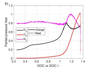
Fig. 4 Partial pressures during charging and later overcharging the battery module vs. (a) time (b) DOC or SOC
