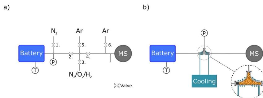
Fig. 1 Schematic presentation of the two different experimental setups. (a) The sampler setup, where valves enabled to sample the battery gas phase once per cycle. (b) The microcapillary setup, where gas is continuously sampled using a microcapillary. The gas is cooled and dried before sampled by the capillary to avoid water condensation and clogging of the system.
