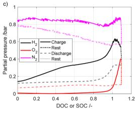
Fig. 3 Partial pressures measured using the (a) microcapillary setup, vs. time; (b) sampler setup vs. time; (c) microcapillary setup, vs. DOC/SOC.
