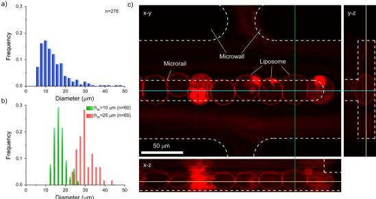
Fig. 6 Size distributions of (a) prepared and (b) trapped liposomes. Liposomes were trapped using the microrail devices with different main channel heights of 10 (green) and 25  $\mu$ m (red). The mean diameters and coefficients of variation of trapped liposomes using microrail devices with 10 and 25  $\mu$ m channel heights were 15.6  $\mu$ m, 9.7%, 28.5  $\mu$ m, and 17.5%, respectively. (c) An orthogonal image of the trapped and aligned liposomes under the microrail.
