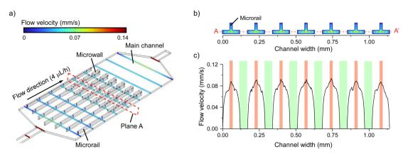
Fig. 4 (a) Flow distribution in the microrail device. The height of the main channel and the height and width of the microrails were 25, 50, and 20  $\mu$ m, respectively. (b) The distribution of flow velocity on the plane A in (a). (c) Flow velocity on the A–A' line in (b) ( $z=12.5~\mu$ m). Orange and green regions show the places where microrails and microwalls were constructed, respectively.
