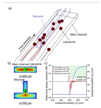
Fig. 3 (a) Trajectories of liposomes with 15  $\mu$ m diameter at a flow velocity of 0.1 mm s<sup>-1</sup>. (b) Cross-sectional views of the microrail channel at x=300 and 700  $\mu$ m. The liposome moved in the *z*-direction. (c) Drag forces on the liposomes and *z*-positions of the liposomes depending on the *x* position of liposomes flowing the microchannels with and without the microrail.
