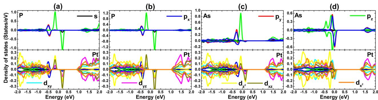
Fig. 11 Projected density of states of impurity and its neighboring Pt atom in (a)  $P_S$ , (b)  $P_{Se}$ , (c)  $As_S$ , and (d)  $As_{Se}$  system.
