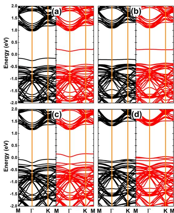
Fig. 9 Spin-resolved band structure (the Fermi level is set to 0 eV; spin-up: black curves; spin-down: red curves) of (a)  $\text{P}_{\text{S}}$ , (b)  $\text{P}_{\text{Se}}$ , (c)  $\text{As}_{\text{S}}$ , and (d)  $\text{As}_{\text{Se}}$  system.
