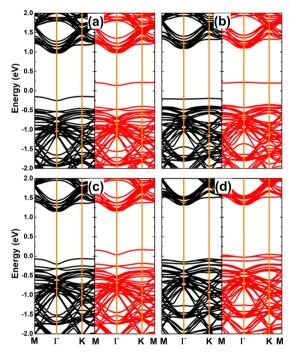
Fig. 9 Spin-resolved band structure (the Fermi level is set to 0 eV; spin-up: black curves; spin-down: red curves) of (a)  $P_{S}$ , (b)  $P_{Se}$ , (c)  $As_{S}$ , and (d)  $As_{Se}$  system.
