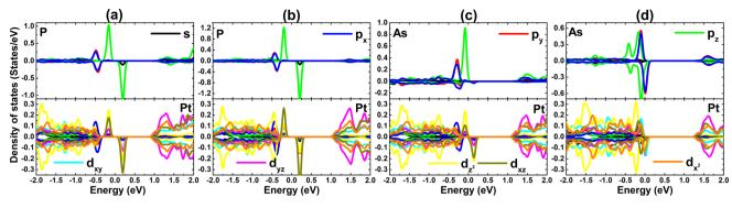
Fig. 11 Projected density of states of impurity and its neighboring Pt atom in (a) P<sub>Sr</sub>, (b) P<sub>Se</sub>, (c) As<sub>S</sub>, and (d) As<sub>Se</sub> system.
