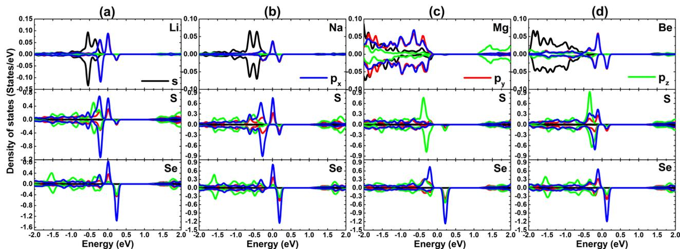
Fig. 8 Projected density of states of impurity and its neighboring S/Se atoms in (a)  $\text{Li}_{\text{Pt}}$ , (b)  $\text{Na}_{\text{Pt}}$ , (c)  $\text{Be}_{\text{Pt}}$ , and (d)  $\text{Mg}_{\text{Pt}}$  system.
