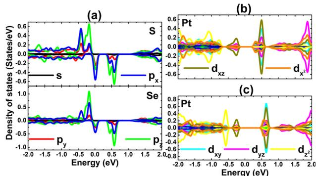
Fig. 5 Projected density of states of atoms closest to the defect site in PtSe monolayer with (a) single Pt vacancy, (b) single S vacancy, and (c) single Se vacancy.
