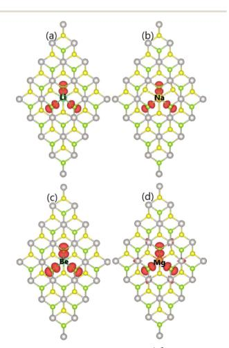
Fig. 7 Spin density (iso-surface value: 0.005 e Å<sup>-3</sup>) in (a) Li<sub>Pt</sub>, (b) Na<sub>Pt</sub>, (c) Be<sub>Pt</sub>, and (d) Mg<sub>Pt</sub> system.
