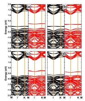
Fig. 6 Spin-resolved band structure (the Fermi level is set to 0 eV; spin-up: black curves; spin-down: red curves) of (a)  $Li_{Pt}$ , (b)  $Na_{Pt}$ , (c)  $Be_{Pt}$ , and (d)  $Mg_{Pt}$  system.
