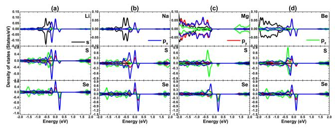
Fig. 8 Projected density of states of impurity and its neighboring S/Se atoms in (a) Li<sub>Pt</sub>, (b) Na<sub>Pt</sub>, (c) Be<sub>Pt</sub>, and (d) Mg<sub>Pt</sub> system.
