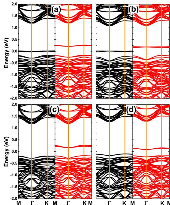
Fig. 6 Spin-resolved band structure (the Fermi level is set to 0 eV; spin-up: black curves; spin-down: red curves) of (a) Li<sub>Pt</sub>, (b) Na<sub>Pt</sub>, (c) Be<sub>Pt</sub>, and (d) Mg<sub>Pt</sub> system.
