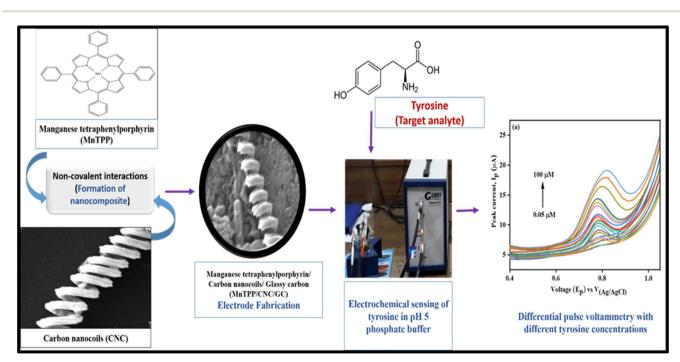
Fig. 1 Graphical representation of CNC/MnTPP/GC modified sensor for the electrochemical detection of tyrosine.
