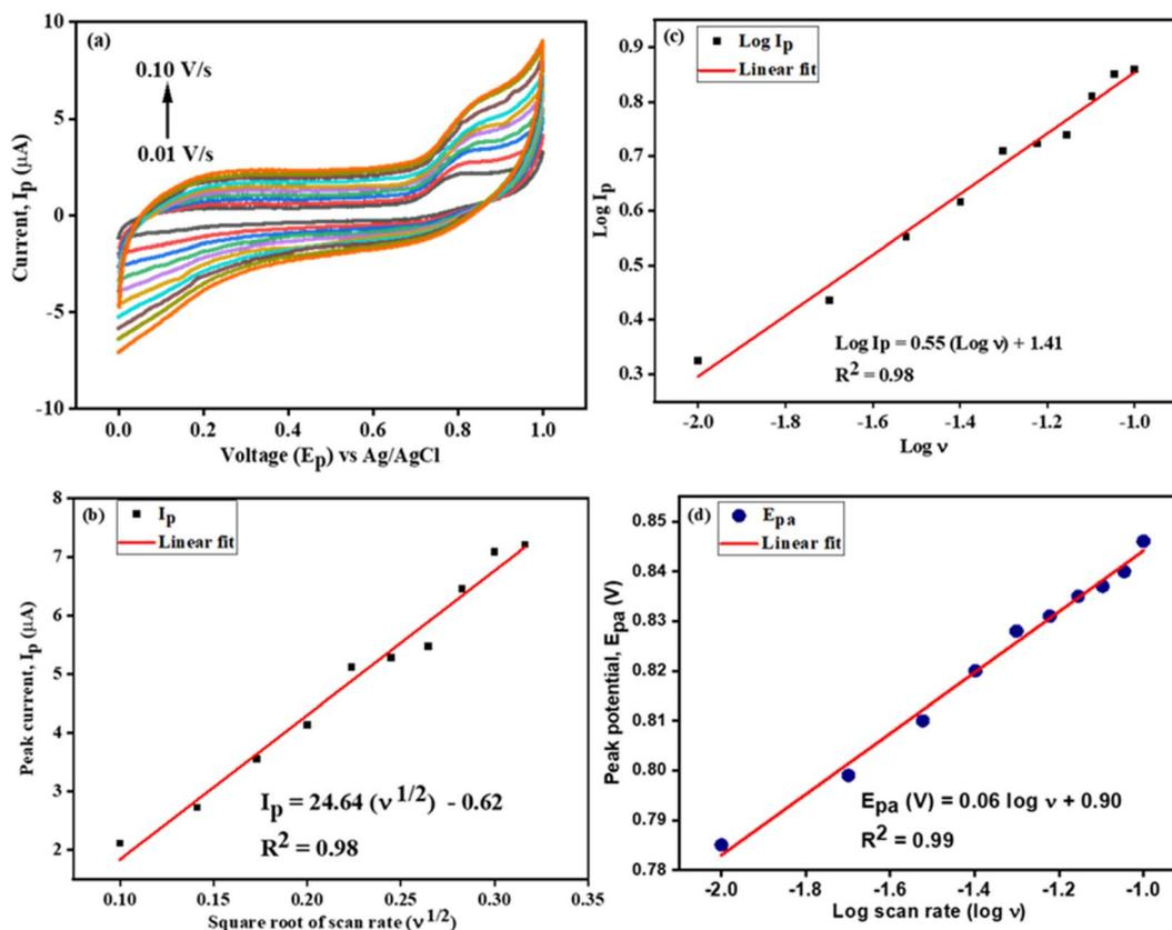
Fig. 9 (a) Effect of scan rate on CNC/MnTPP/GC in 100  $\mu\text{M}$  tyrosine at pH 5.0 (b) calibration plot for change of current as a function of square root of scan rate, (c)  $\log I_p$  vs.  $\log v$  and (d)  $E_{pa}$  vs.  $\log v$ .
