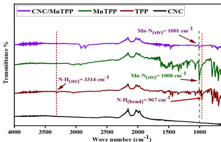
Fig. 2 FTIR of CNC/MnTPP, MnTPP, TPP, and CNC.
