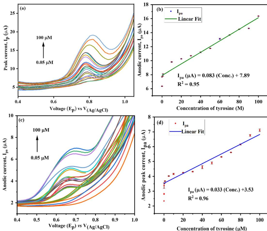
Fig. 11 DPV depicting the influence of varying concentrations of tyrosine (0.05 to 100  $\mu$ M) on CNC/MnTPP/GC in 0.1 M PBS at (a) pH 5.0, (b) calibration plot at pH 5, (c) DPV at pH 7.4 and (d) calibration plot at pH 7.4.
