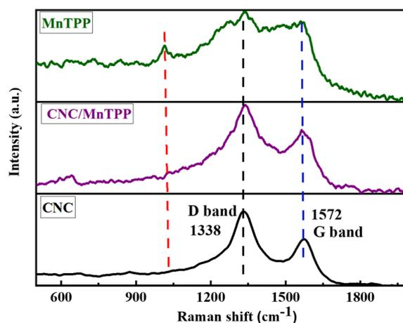
Fig. 3 Raman analysis of MnTPP, CNC/MnTPP, and CNC.
