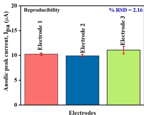
Fig. 13 Reproducibility studies of CNC/MnTPP/GC sensor in 100  $\mu\text{M}$  tyrosine solution (pH 5).
