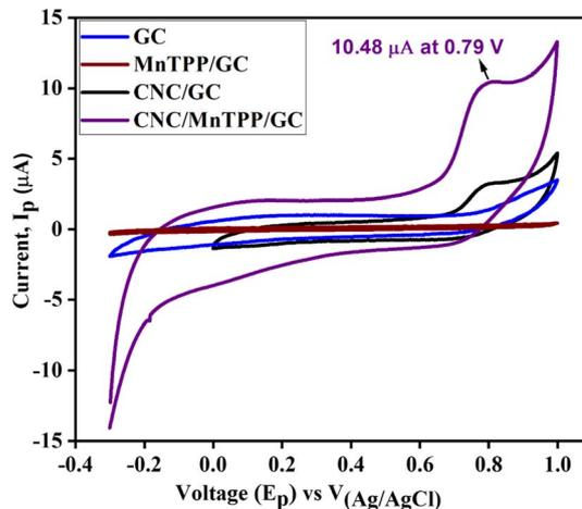
Fig. 7 Cyclic voltammograms of GC, MnTPP/GC, CNC/GC, and CNC/MnTPP/GC in 100  $\mu\text{M}$  tyrosine in 0.1 M PBS (conditions; scan rate = 0.05  $\text{V s}^{-1}$ ; pH 5).
