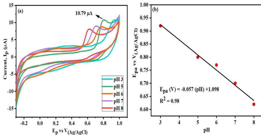
Fig. 8 (a) Effect of pH 3, 5, 6, 7 and 8 on CNC/MnTPP/GC in 100  $\mu\text{M}$  tyrosine in 0.1 M PBS and (b) calibration plot for change in peak potential as well as peak current as a function of change in pH (pH 3, 5, 6, 7 and 8).
