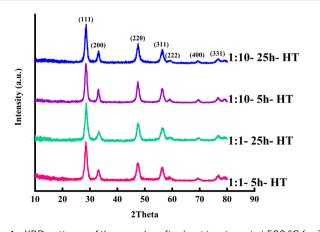
Fig. 4  $\,$  XRD patterns of the samples after heat treatment at 500  $^{\circ}$ C for 3 hours.
