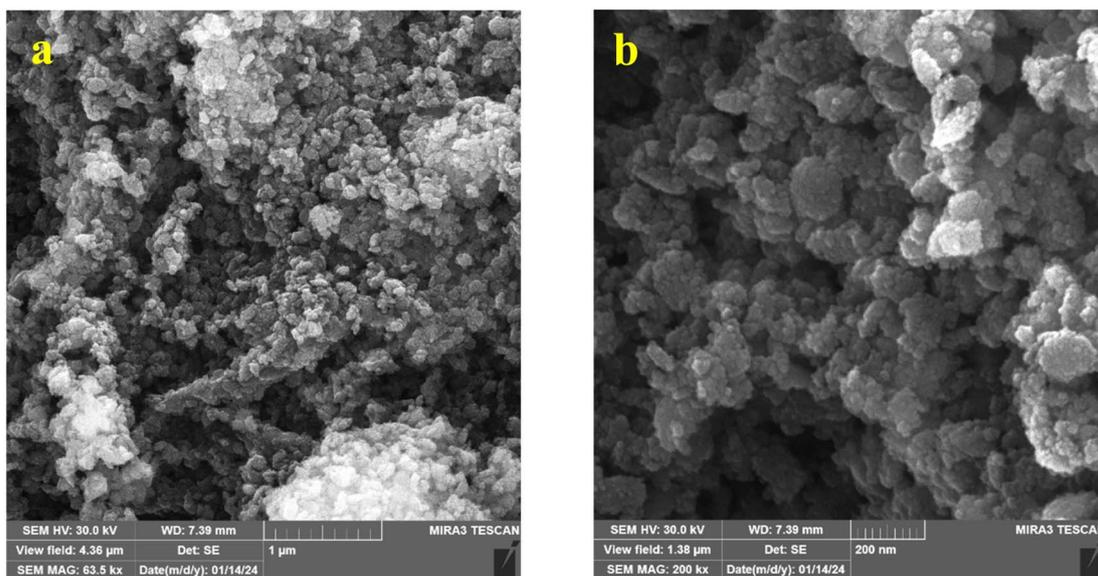
Fig. 2 SEM images of sample 1:10-25 h: (a) magnification of 30kx and (b) magnification of 200kx.
