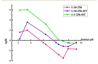
Fig. 9  $\Delta$ pH versus initial pH to determine pH<sub>PZC</sub>.
