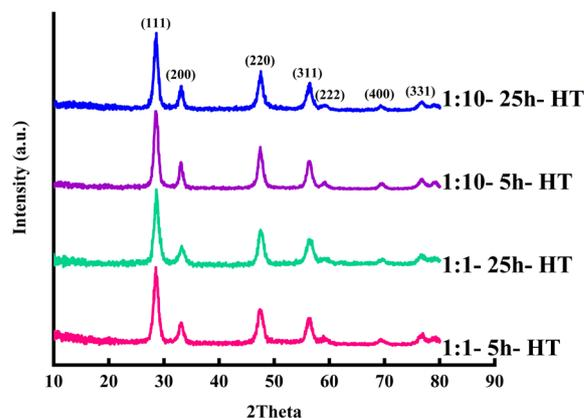
Fig. 4 XRD patterns of the samples after heat treatment at 500 °C for 3 hours.
