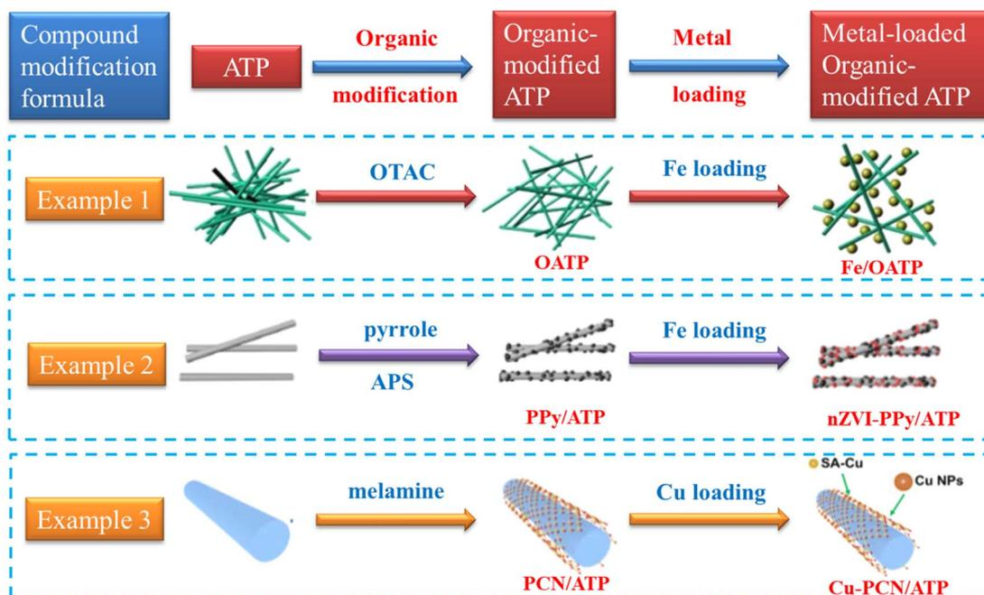
Fig. 4 Compound modification processes of ATP.<sup>122,124,126</sup> Copyright 2024, Elsevier.
