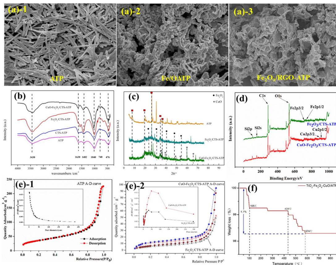
Fig. 5 Characterizations of attapulgite composite materials (a) SEM graphs (b) FT-IR curves, (c) XRD curves, (d) XPS, (e) BET A-D curves and (f) TG curve.<sup>103,114,122,128</sup> Copyright 2024, MDPI.
