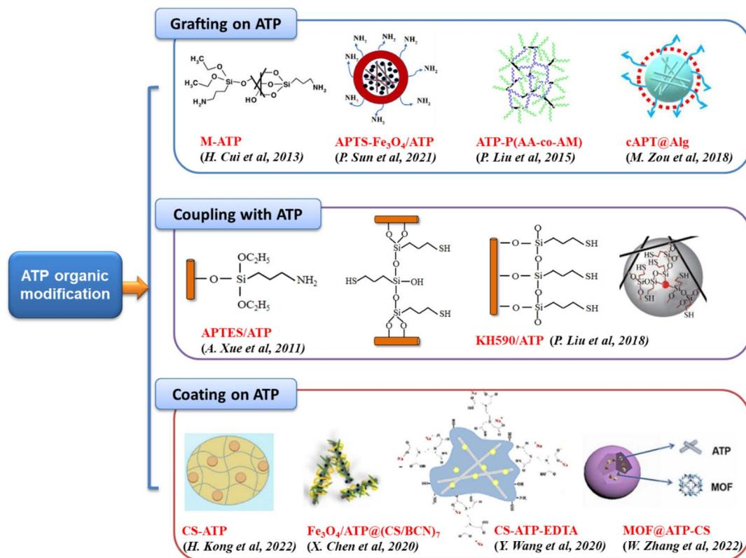
Fig. 2 ATP organic modification methods.<sup>75,86–94</sup> Copyright 2024, Elsevier.
