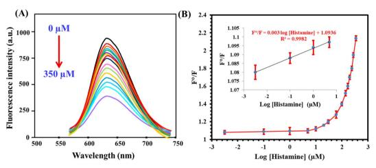
Fig. 4 (A) The influence of histamine addition  $(0.003-350 \mu M)$  on the fluorescence emission of the fluorescent probe. (B) Corresponding calibration plot.
