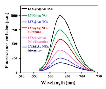
Fig. 3 The fluorescence responses of different probes in the presence and absence of histamine (350  $\mu$ M).
