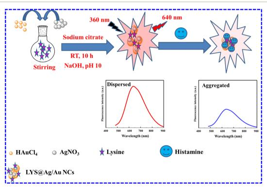
Scheme 1 Steps for preparation of LYS@Ag/Au NCs and fluorometric determination of histamine.
