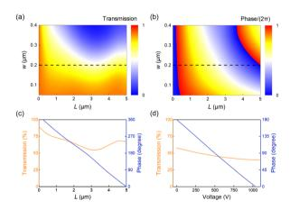
Fig. 2 Design of on-chip unit structure. Simulated (a) transmission and (b) phase shift of the device unit structure as a function of L and w. The black dashed lines represent the parameter w=200 nm. (c) Simulated transmission (orange curve) and phase shift (blue curve) versus slot length L, with w=200 nm. (d) Simulated transmission (orange curve) and phase shift (blue curve) with voltage from 0 to 1100 V, with L=2714.5 nm, W=200 nm.
