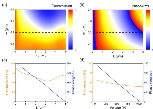
**Fig. 2** Design of on-chip unit structure. Simulated (a) transmission and (b) phase shift of the device unit structure as a function of  $L$  and  $w$ . The black dashed lines represent the parameter  $w = 200$  nm. (c) Simulated transmission (orange curve) and phase shift (blue curve) versus slot length  $L$ , with  $w = 200$  nm. (d) Simulated transmission (orange curve) and phase shift (blue curve) with voltage from 0 to 1100 V, with  $L = 2714.5$  nm,  $w = 200$  nm.
