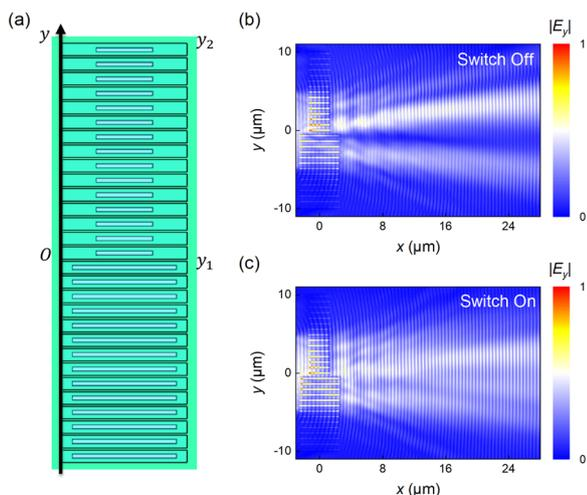
Fig. 3 Simulated results of the oracle metasurface. (a) Schematic structure of the oracle metasurface. The electric field distribution  $|E_y|$  in LN layer, when the applied voltage is (b) switch off, and (c) switch on.
