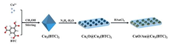
Scheme 1 Schematic illustration of the synthesis process of CuO/Au@Cu<sub>3</sub>(BTC)<sub>2</sub>.
