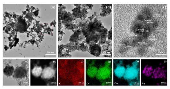
Fig. 2 Morphology characterizations of the  $CuO/Au@Cu_3(BTC)_2$  sample. (a) TEM image, (b) partial magnification in (a), (c) HRTEM image, and (d–i) EDX-mapping images.
