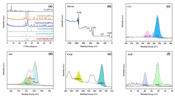
Fig. 1 (a) XRD patterns of the as-prepared samples, (b) survey, (c) C1s, (d) O1s, (e) Cu2p, and (f) Au4f XPS spectra of the CuO/Au@Cu<sub>3</sub>(BTC)<sub>2</sub> sample.
