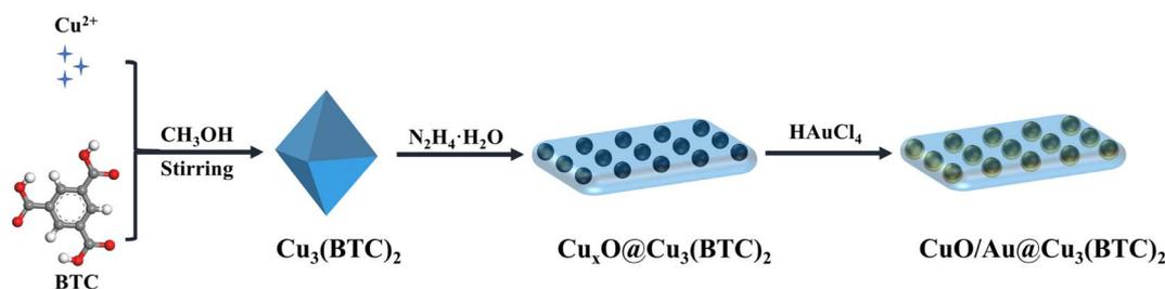
Scheme 1 Schematic illustration of the synthesis process of CuO/Au@Cu<sub>3</sub>(BTC)<sub>2</sub>.
