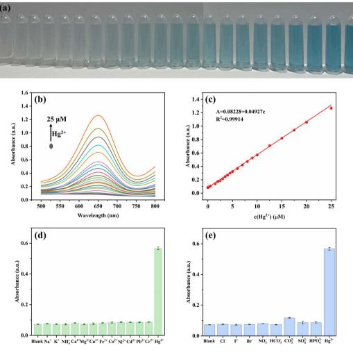
Fig. 4 (a) Photo and (b) UV-vis spectra of the colorimetric response of CuO/Au@Cu<sub>3</sub>(BTC)<sub>2</sub>-TMB to different concentrations of Hg<sup>2+</sup>. (c) Calibration curve of  $A_{652}$  versus concentration of Hg<sup>2+</sup>, (d) and (e) are selectivity responses of CuO/Au@Cu<sub>3</sub>(BTC)<sub>2</sub>-TMB to Hg<sup>2+</sup> (10  $\mu$ M) and the interference ions (0.1 mM).
