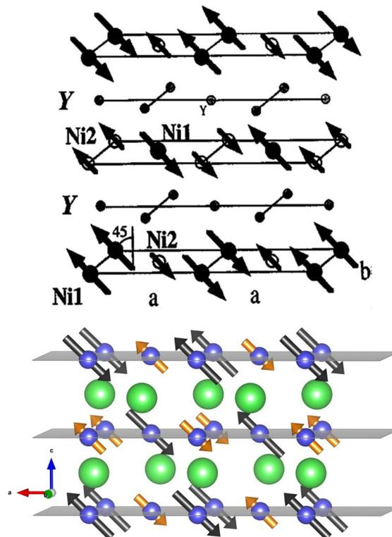
Fig. 3 Antiferromagnetic ordering of the  $\text{YNiO}_3$  perovskite at room temperature obtained by Alonso *et al.*<sup>5</sup> (top) compared to the present calculated result produced with the VESTA program<sup>10</sup> (bottom).
