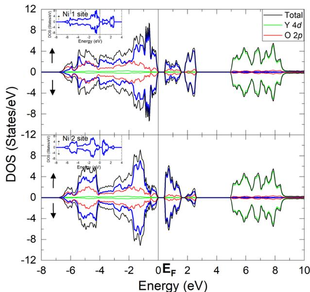
Fig. 2 Projected density of states (DOS) of the  $\text{YNiO}_3$  compound separated into the Ni1 (upper panel) and the Ni2 (lower panel) nonequivalent sites. The DOS in each panel are split in the majority (above) and minority (below) spin bands. The Fermi level separates the occupied states in the valence band from the unoccupied states in the conduction band.
