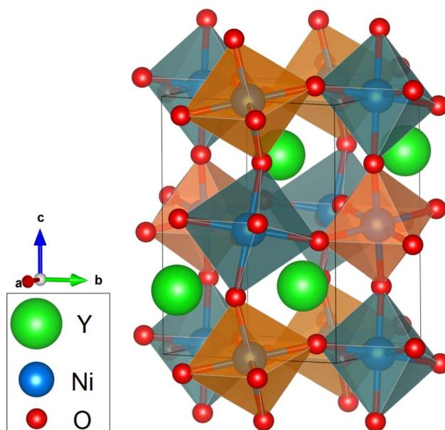
Fig. 1 Schematic VESTA representation of the crystalline structure of  $\text{YNiO}_3$  with shorter and larger Ni–O bonds indicated by orange and dark green octahedra, respectively.<sup>10</sup>
