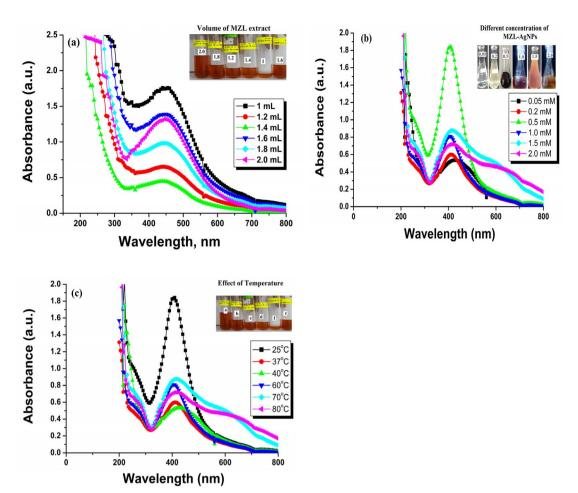
Fig. 6 Optimization of the green synthesized AqNP-MZL: effect of volume of MZL extract (a), effect of concentration of the green synthesized AgNP-MZL (b) and effect of temperature (c).
