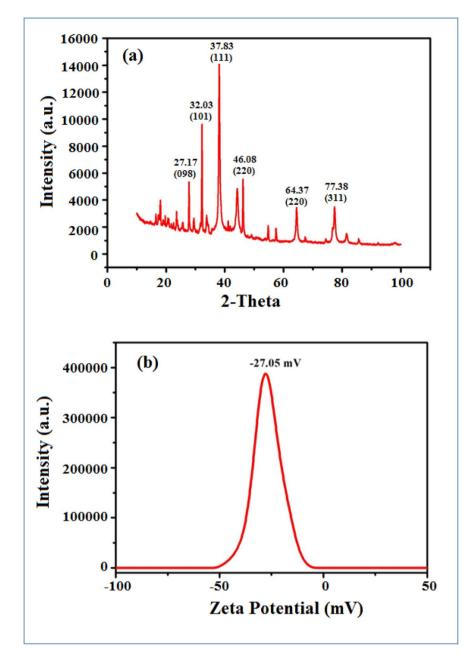
Fig. 4 XRD pattern (a) and zeta potential (b) of green synthesized AgNPs by MZL extract.
