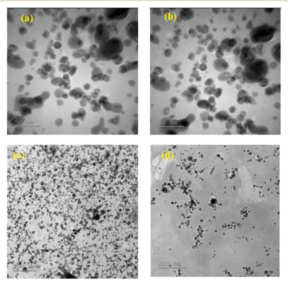
Fig. 2 Two magnifications of  $\times$ 50 and  $\times$ 200 nm of the TEM image of (a and b) green synthesized AgNP-MZL and (c and d) green synthesized AgNP-MZL binding with STR antibiotic, respectively.
