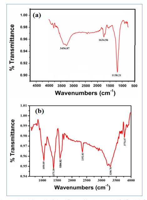
Fig. 5 FTIR spectra of green synthesized dispersed AgNPs from MZL extract (a) and aggregated AgNP–MZL with AMG antibiotic (STR) (b).
