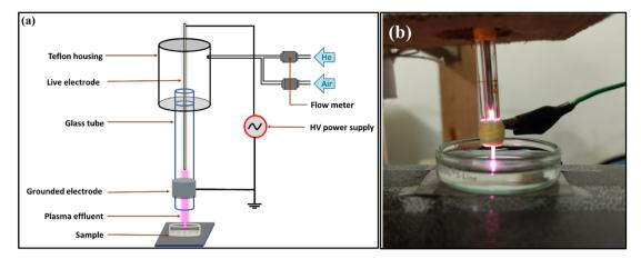
Fig. 2 Schematic diagram of the experimental setup (a); photograph of the lab-developed plasma jet setup (b).
