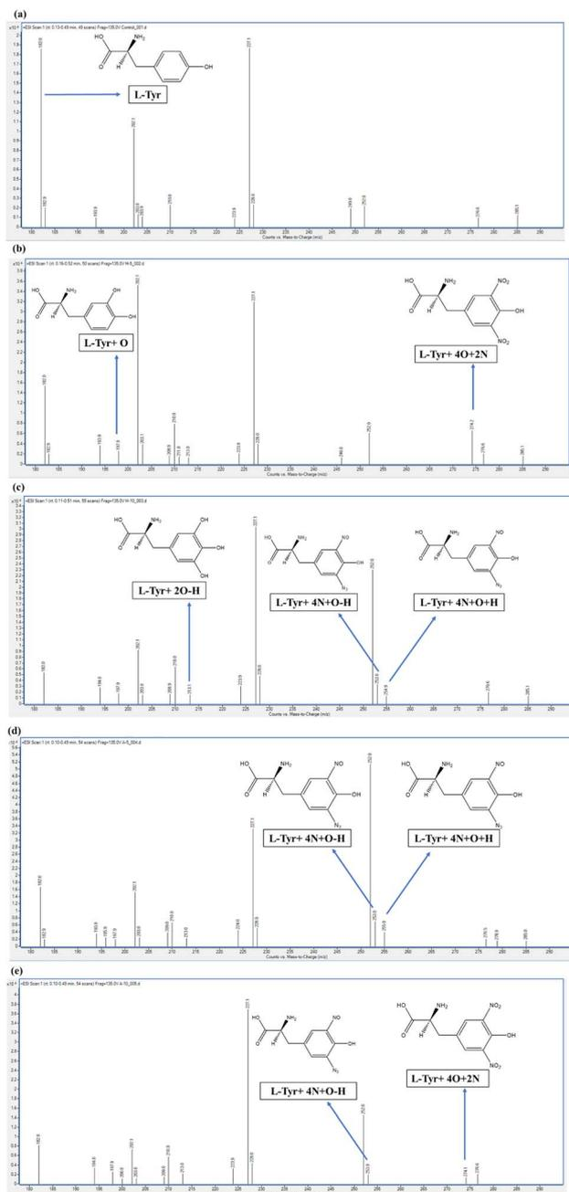
Fig. 4 LC-QQQ-mass spectra of the aqueous solution of protonated tyrosine sample  $[(\text{Tyr})\text{H}^+]$  (a), helium-treated L-tyrosine samples at 5 min and 10 min (b and c) and He-air treated L-Tyr samples at 5 min and 10 min (d and e).
