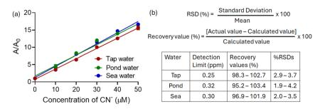
Fig. 5 (a) Changes in the absorbance of  $\bf 1$  at 440 nm upon addition of CN $^-$  ion in real-life samples (CH $_3$ CN-H $_2$ O, 7:3 v/v). (b) Quantitative analysis of CN $^-$  ion in real-life water samples.
