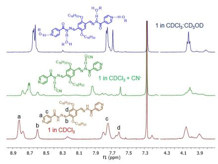
Fig. 4 Partial  $^{1}$ H-NMR spectra of 1 with CN $^{-}$  ion in CDCl<sub>3</sub> medium and also in presence of CD<sub>3</sub>OD (CDCl<sub>3</sub>: CD<sub>3</sub>OD = 5:1).
