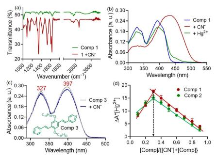
Fig. 3 (a) FT-IR spectra of 1 with CN $^-$  ion. (b) UV-visible spectra of 1 (10  $\mu$ M) with CN $^-$  ion (100  $\mu$ M) and subsequently treated with Hg $^{2+}$  (50  $\mu$ M). (c) UV-visible spectra of 3 (10  $\mu$ M) with CN $^-$  ion (100  $\mu$ M) in CH $_3$ CN $^-$ water (7:3) medium. (d) Job's plot analysis shows 1:2 binding stoichiometry between probe molecules (1, 2) and CN $^-$  ion.
