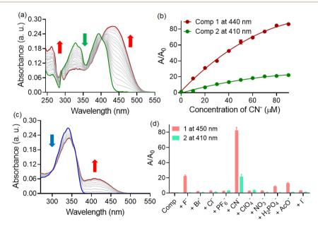
Fig. 2 UV-visible titrations of (a) 1 (c) 2 (10  $\mu$ M) with CN<sup>-</sup> ion (100  $\mu$ M) in CH<sub>3</sub>CN-water (7 : 3) medium. (b) Change in absorbance of compounds 1 and 2 (10  $\mu$ M) with CN<sup>-</sup> ion (0–100  $\mu$ M) in CH<sub>3</sub>CN-water (7 : 3) medium. (d) Change in absorbance of 1 and 2 (10  $\mu$ M) with different anions (100  $\mu$ M) in CH<sub>3</sub>CN-water (7 : 3) medium.
