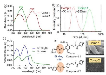
Fig. 1 (a) UV-visible spectra of 1 and 2 (10  $\mu$ M) in CH<sub>3</sub>CN-water (7 : 3) medium. (b) Dynamic light scattering experiment of 1 and 2 (10  $\mu$ M) in CH<sub>3</sub>CN-water (7 : 3) medium. (c) UV-visible spectra of 1 (10  $\mu$ M) in water and CH<sub>3</sub>CN medium. (d) FESEM images and structure of compound 1 and 2.
