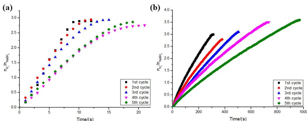
Fig. 9 Reusability assay for NaBH<sub>4</sub> hydrolysis using 34.45 μmol of PtNPs (a) and NiNPs (b) over 100 mg of niobic acid (0.5 mmol of NaBH<sub>4</sub> in the final volume of 2 mL of type II+ water). The catalyst was washed and vacuum-dried before each reuse (24 ± 1 °C).
