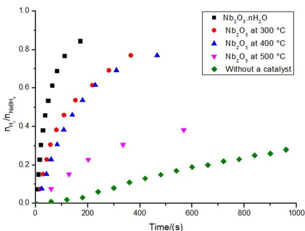
Fig. 3 Hydrogen production ratio with respect to the substrate (0.5 mmol of NaBH<sub>4</sub> in the final volume of 21 mL of type II+ water at 27.0 ± 1.0 °C) in the reactions catalyzed by 100 mg of niobic acid or its heat-treated counterparts (at 300, 400, and 500 °C).
