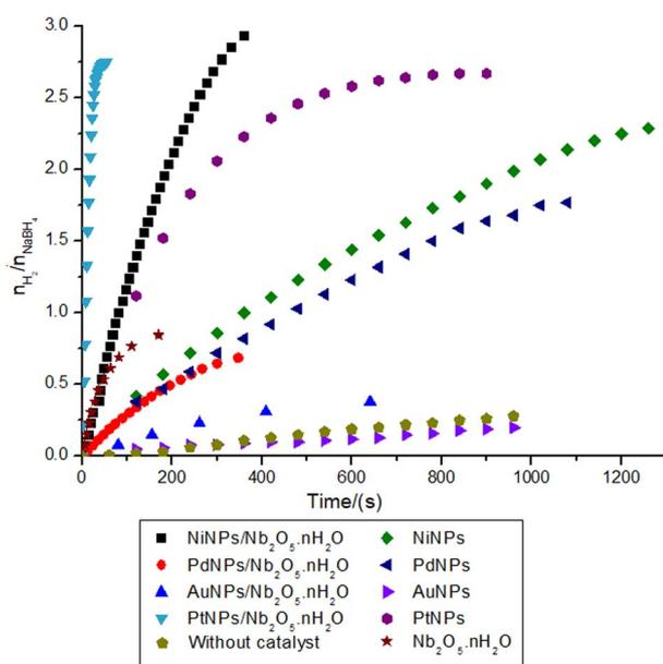
Fig. 4 Hydrogen production ratio with respect to the substrate (0.5 mmol of NaBH<sub>4</sub> in the final volume of 21 mL of type 1 water at 27.0 ± 0.5 °C) in the reactions catalyzed by niobic acid-supported and non-supported metal nanocatalyst (Ni, Pd, Au, or PtNPs).
