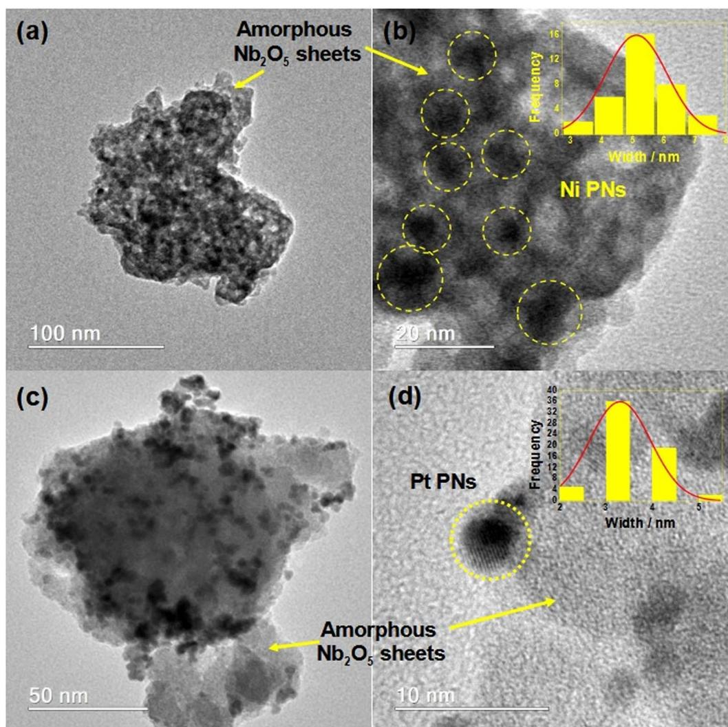
**Fig. 2** TEM images of the (a and b) NiNPs/Nb<sub>2</sub>O<sub>5</sub>·*n*H<sub>2</sub>O, inset: NiNPs size distribution. (c and d) PtNPs/Nb<sub>2</sub>O<sub>5</sub>·*n*H<sub>2</sub>O, inset: PtNPs size distribution.
