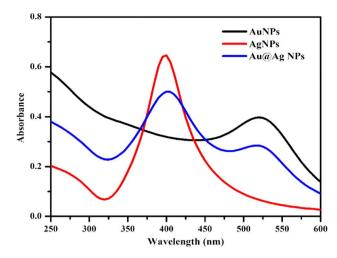
Fig. 1 UV-visible spectra of AgNPs, AuNPs and Au@Ag NPs.
