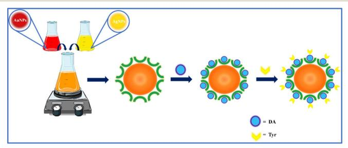
Scheme 4 Interaction mechanism of Au@Ag NPs with DA and Tyr.
