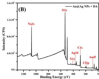
Fig. 4 XPS spectra of (A) Au@Ag NPs and (B) Au@Ag NPs with dopamine.
