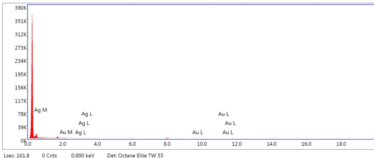
Fig. 3 EDX spectra of Au@Ag NPs.
