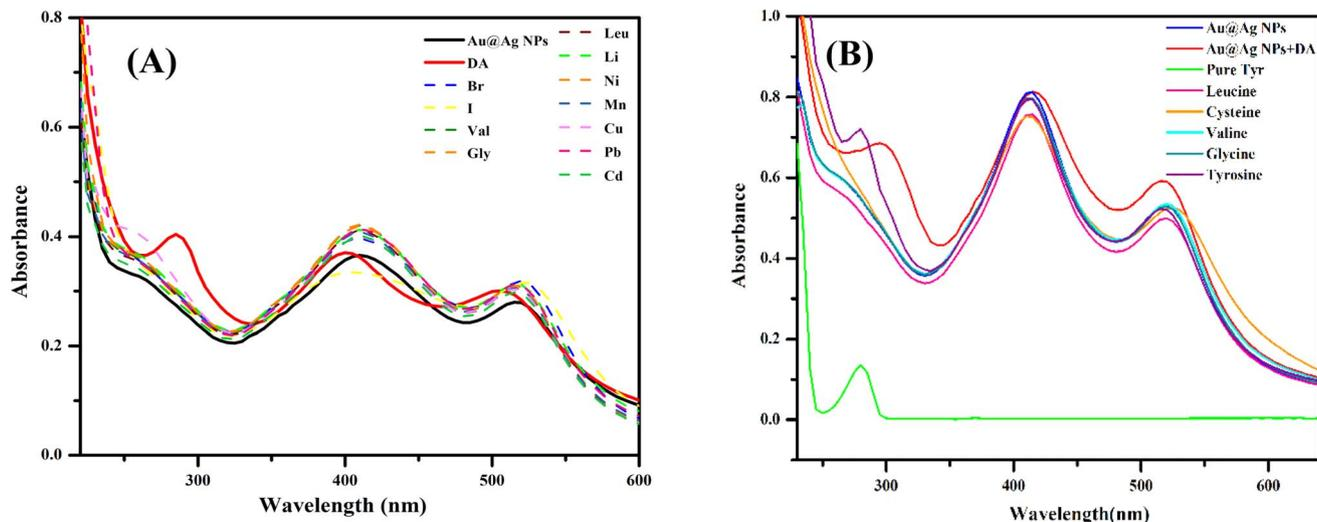
Fig. 7 UV-visible spectra showing the (A) effect of different interfering substances on the Au@Ag NPs–DA system and (B) effect of different biomolecules on the interaction of the Au@Ag NPs–DA system with Tyr.
