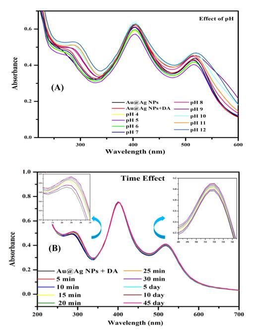
Fig. 8 Optimization of the Au@Ag NPs-DA system: (A) different pH values and (B) time periods.
