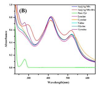
Fig. 7 UV-visible spectra showing the (A) effect of different interfering substances on the Au@Ag NPs-DA system and (B) effect of different biomolecules on the interaction of the Au@Ag NPs-DA system with Tyr.
