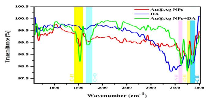
Fig. 5 FTIR spectra of Au@AgNPs, dopamine and Au@Ag NPs after the addition of dopamine.
