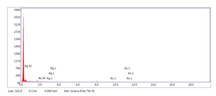
Fig. 3 EDX spectra of Au@Ag NPs.
