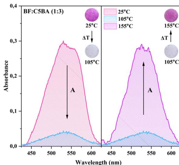
Fig. 6 Absorption spectra of BF : C5BA (1 : 3), measured at 25 °C, 105 °C, and 155 °C.
