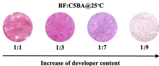
Fig. 2 Diagram presenting composition optimization of BF : C5BA-based materials.
