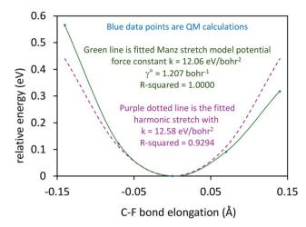
Fig. 5 Quantum-mechanically-computed Born-Oppenheimer potential energy curve for the C-F bond stretch in the  $C_6F_6$  molecule. Fitted harmonic and Manz stretch model potentials are shown for comparison.
