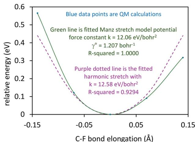
Fig. 5 Quantum-mechanically-computed Born–Oppenheimer potential energy curve for the C–F bond stretch in the  $\text{C}_6\text{F}_6$  molecule. Fitted harmonic and Manz stretch model potentials are shown for comparison.
