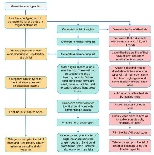
Fig. 5 Flowchart for generating lists of stretch types and instances, angle types and instances, and dihedral types and instances.
