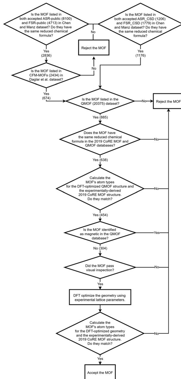
Fig. 4 Crystal geometry verification procedure workflow.
