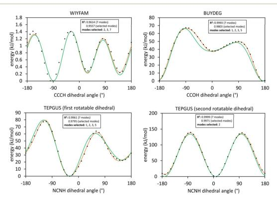
Fig. 13 Potential energy curves for rigid torsion scans of rotatable dihedrals. In each panel, the black dots show the quantum mechanical energy obtained from single-point DFT\_with\_dispersion calculations. The orange curve illustrates the fitted model using all 7 modes, while the green curve shows the fitted model using only the smart-selected modes.
