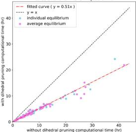
Fig. 24 Parity plot showing computational time for flexibility parameters calculation when the flexibility model was constructed with dihedral pruning compared to without dihedral pruning. These computational times include optimizing force constant values, computing statistics for the training datasets, and computing statistics for the validation datasets. These computational times do not include the times for quantum chemistry calculations to prepare the training and validation datasets.
