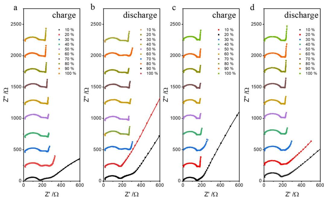
Fig. 5 Nyquist plots of impedance spectra of all-solid-state TFBS based on  $\text{LiCoO}_2/\text{LiPON/Li}$  for (a) charge and (b) discharge processes at different charge–discharge states. TFBS based on  $\text{LiCoO}_2/\text{V}_2\text{O}_5\text{-5 nm/LiPON/Li}$  for (c) charge and (d) discharge processes at different charge–discharge states from 0% to 100% at the interval of 10%. The fitted results are shown as solid lines.
