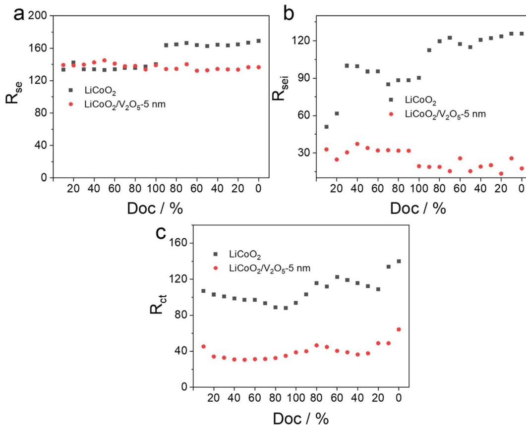
Fig. 6 The variation of impedance (a)  $R_{se}$ , (b)  $R_{sei}$ , and (c)  $R_{ct}$  with different charge–discharge states (depth of charge, doc) from 0% to 100% at the interval of 10% for all-solid-state TFBS based on LiCoO<sub>2</sub>/LiPON/Li and LiCoO<sub>2</sub>/V<sub>2</sub>O<sub>5</sub>-5 nm/LiPON/Li.
