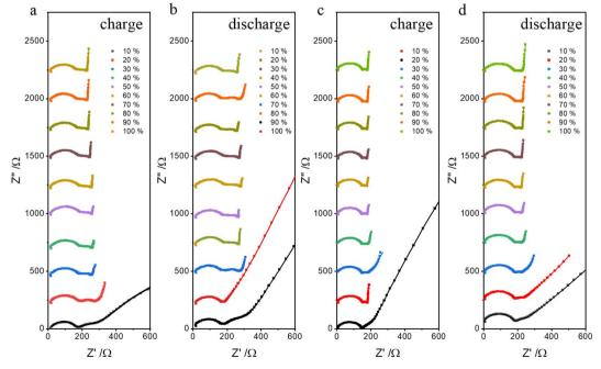
Fig. 5 Nyquist plots of impedance spectra of all-solid-state TFBs based on LiCoO<sub>2</sub>/LiPON/Li for (a) charge and (b) discharge processes at different charge–discharge states. TFBs based on LiCoO<sub>2</sub>/ $V_2O_5$ -5 nm/LiPON/Li for (c) charge and (d) discharge processes at different charge–discharge states from 0% to 100% at the interval of 10%. The fitted results are shown as solid lines.
