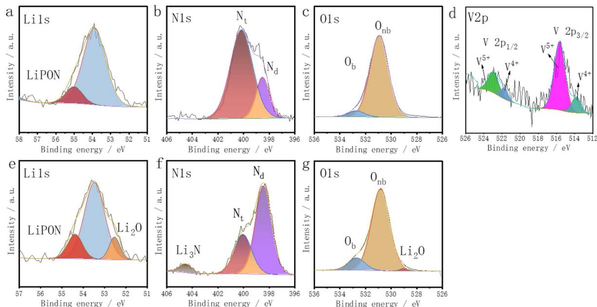
Fig. 2 High-resolution XPS spectra for elemental (a) Li 1s, (b) N 1s, (c) O 1s, and (d) V 2p of the  $\text{LiCoO}_2/\text{V}_2\text{O}_5/\text{LiPON}$  film, and (e) Li 1s (f) N 1s, and (g) O 1s of the  $\text{LiCoO}_2/\text{LiPON}$  film.
