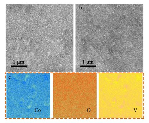
Fig. 1 Representative top-view SEM images for the surface morphology of the as-prepared (a) LiCoO<sub>2</sub> cathode film and (b) LiCoO<sub>2</sub>/V<sub>2</sub>O<sub>5</sub> film. (c) The corresponding EDS 2D mapping for element distributions of Co (blue), O (orange), and V (yellow) in the image of (b) the LiCoO<sub>2</sub>/V<sub>2</sub>O<sub>5</sub> film.
