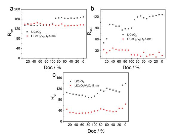
Fig. 6 The variation of impedance (a)  $R_{\rm sei}$ , (b)  $R_{\rm sei}$ , and (c)  $R_{\rm ct}$  with different charge—discharge states (depth of charge, doc) from 0% to 100% at the interval of 10% for all-solid-state TFBs based on LiCoO<sub>2</sub>/LiPON/Li and LiCoO<sub>2</sub>/V<sub>2</sub>O<sub>5</sub>-5 nm/LiPON/Li.
