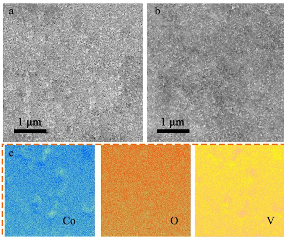
Fig. 1 Representative top-view SEM images for the surface morphology of the as-prepared (a)  $\text{LiCoO}_2$  cathode film and (b)  $\text{LiCoO}_2/\text{V}_2\text{O}_5$  film. (c) The corresponding EDS 2D mapping for element distributions of Co (blue), O (orange), and V (yellow) in the image of (b) the  $\text{LiCoO}_2/\text{V}_2\text{O}_5$  film.
